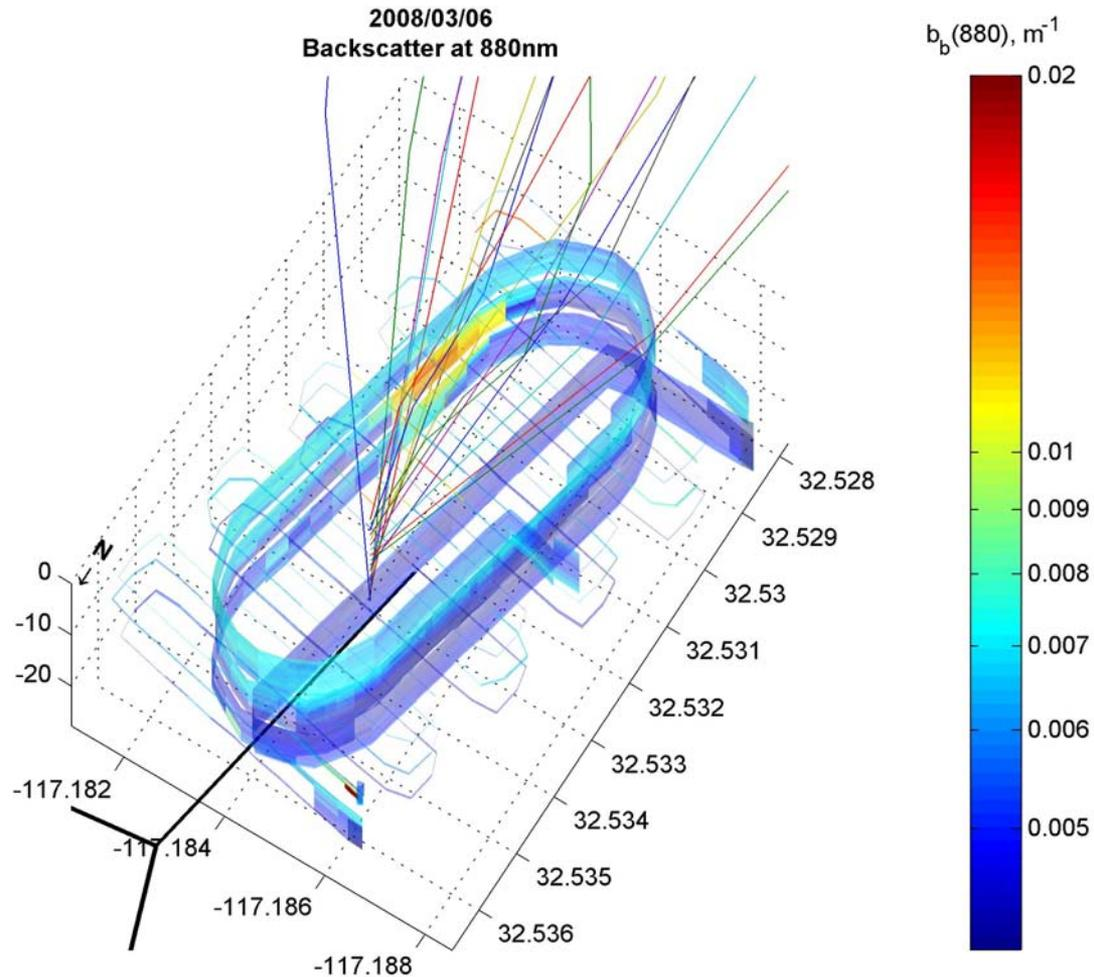
Near-field backscatter measurements at 880 nm shows good correspondence between elevated values ( $>0.01 m^{-1}$ ) and the estimated plume trajectory indicating elevated turbidity associated with the effluent.
