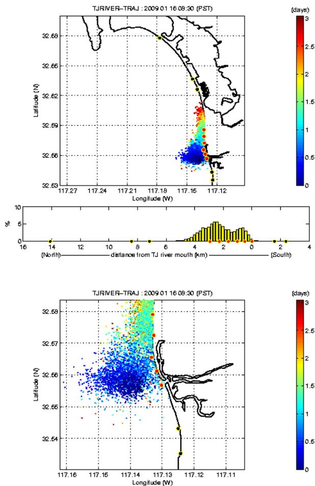
**Figure E.4 Tijuana River Plume Tracking Model**
