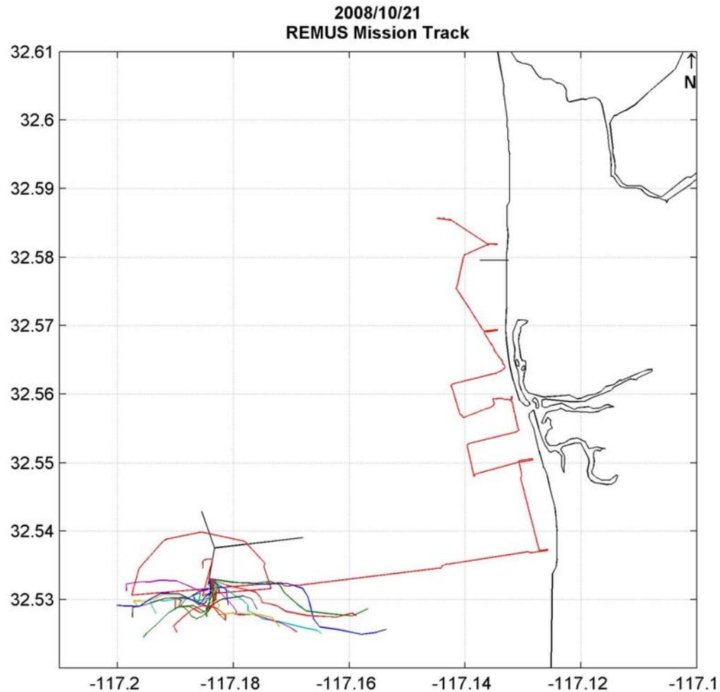
REMUS track (red) and estimated SBOO plume trajectory (colored lines) based on near-realtime velocity profiles measured by the SBOO buoy for a hybrid SBOO-Tijuana River mission.
