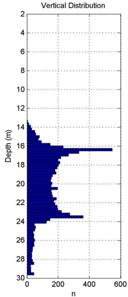
Horizontal and vertical plume distributions based on thresholding by the plumes' signature salinity value. The number of samples satisfying the threshold criteria for a given horizontal or vertical bin is given by 'n'.
