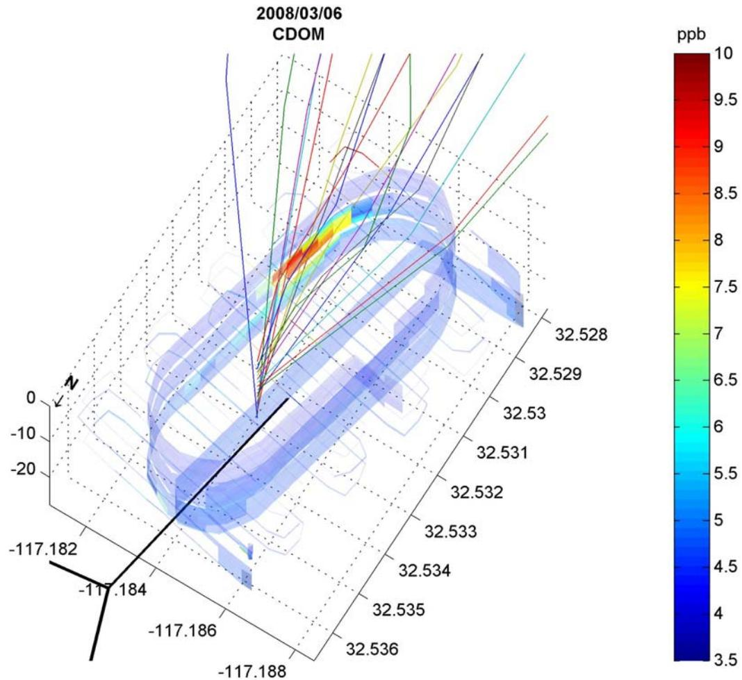
Near-field CDOM measurements shows good correspondence between elevated values (> 7 ppb) and the estimated plume trajectory.
