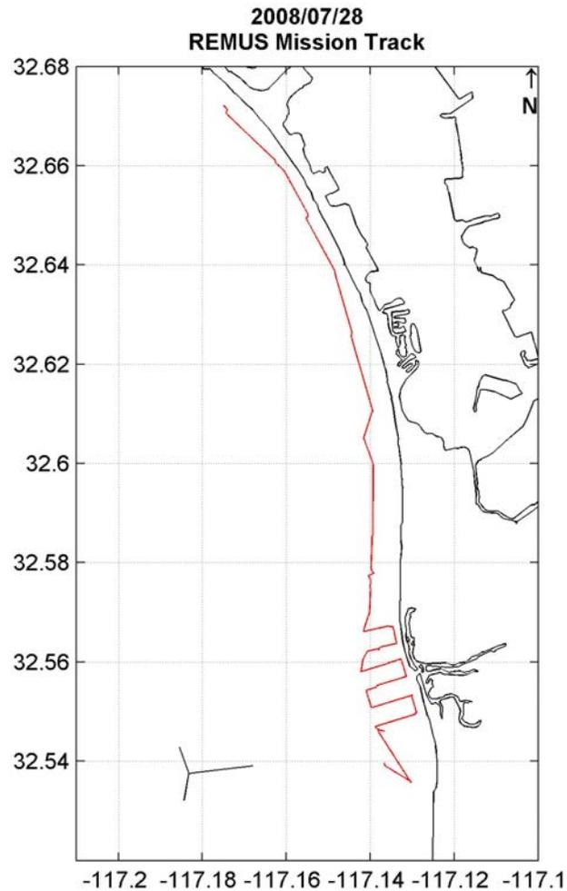
REMUS track (red) for a nearshore 'baseline' mission aimed at revealing background values for physical and optical parameters during dry weather and southward alongshore flow.
