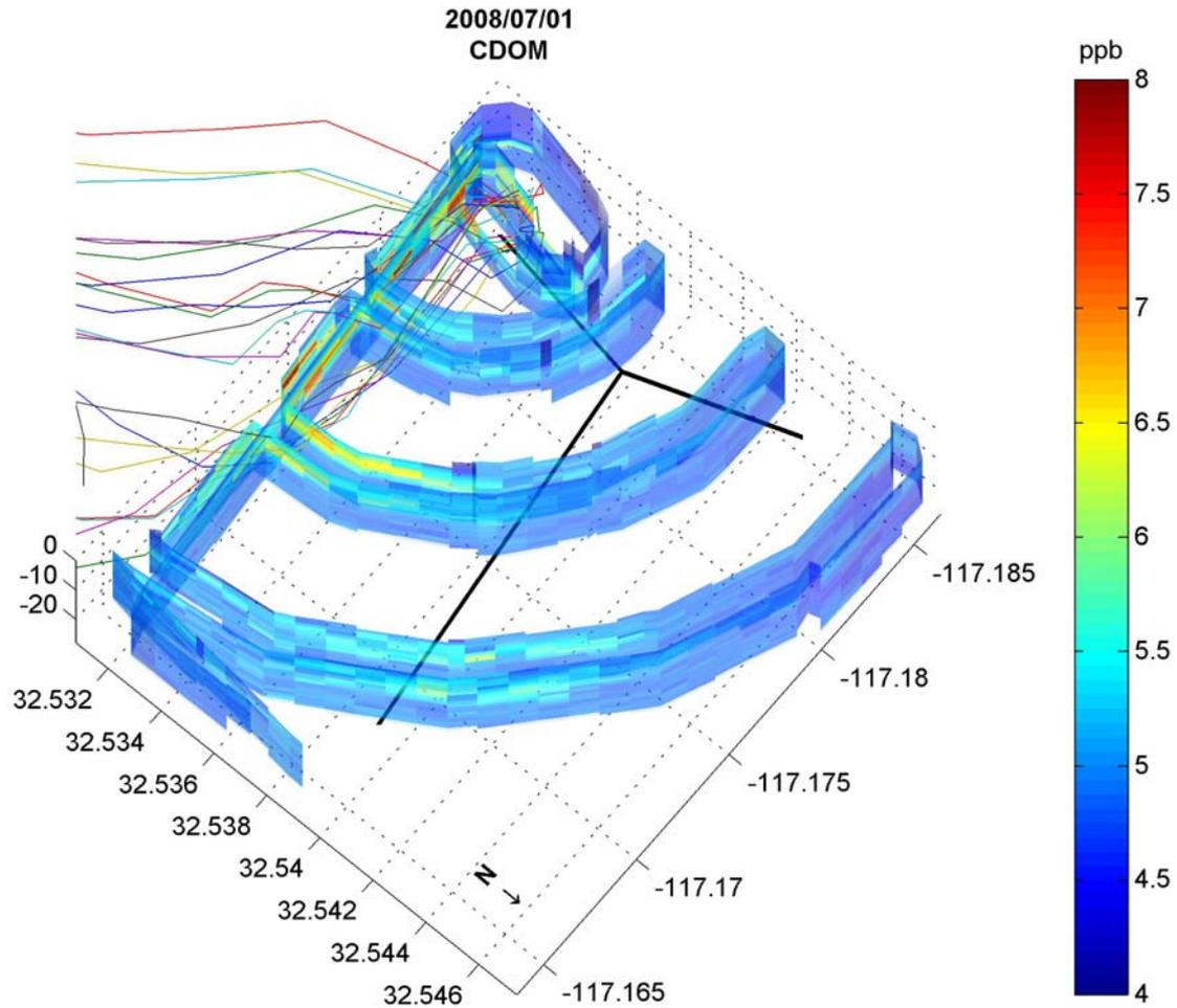
Elevated CDOM measurements ( $> 5.5$  ppb) show good correspondence with the estimated SBOO plume trajectory (colored lines) based on near-realtime velocity profiles measured by the SBOO buoy.
