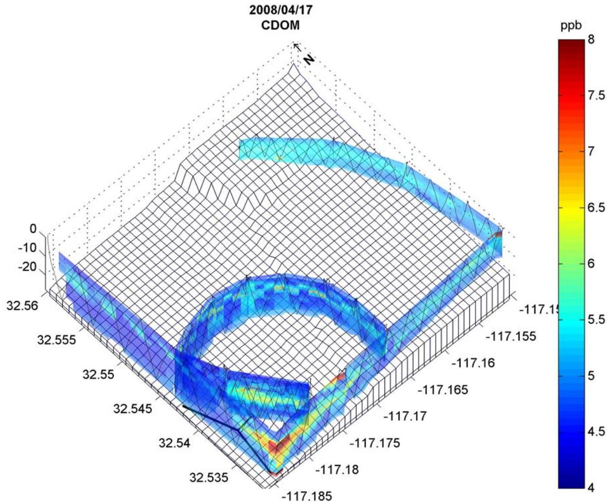
Elevated CDOM values ( $> 5$  ppb) near the outfall toward the south indicate detection of the outfall plume. CDOM values of approximately 5.5 ppb in the northeast are within the kelp forest and are presumably due to elevated biological activity.
