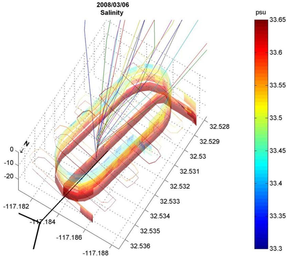
Salinity measurements shown with estimated SBOO plume trajectory (colored lines) based on near-realtime velocity profiles measured by the SBOO buoy. Low salinity near the outfall and northward shows good agreement with the estimated trajectory.
