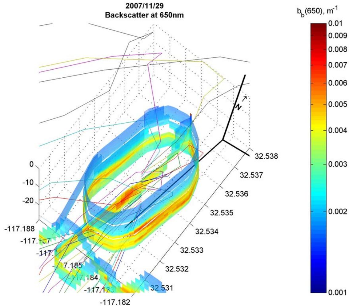
Near-field backscatter measurements at 650nm show good correspondence between elevated values ( $>0.004 \text{ m}^{-1}$ ) and the estimated plume trajectory indicating elevated turbidity associated with the effluent.
