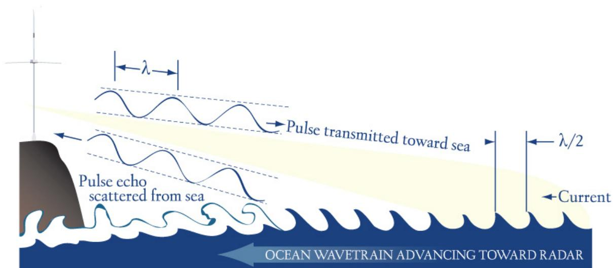
Figure E.3 Representation of HF Radar Technology
