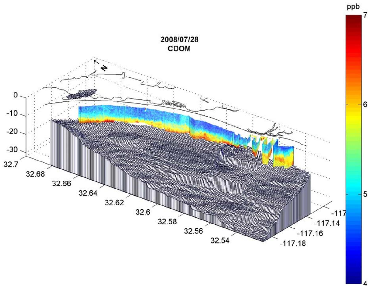
CDOM shows elevated values (>5 ppb) near the surface at the Tijuana River mouth indicating exchange with the estuary during periods of no flow. Elevated values (> 5.5 ppb) near the seafloor may be due to sediment resuspension by currents scouring bottom sediment.
