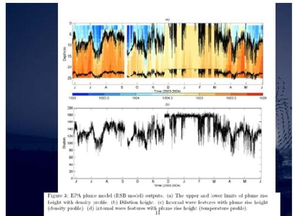
Figure 3: EPA plume model (RSB model) outputs. (a) The upper and lower limits of plume rise height with density profile. (b) Dilution height. (c) Internal wave features with plume rise height (density profile). (d) Internal wave features with plume rise height (temperature profile).
