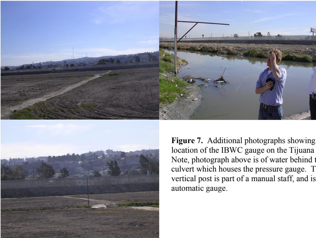
**Figure 7.** Additional photographs showing the location of the IBWC gauge on the Tijuana River. Note, photograph above is of water behind the culvert which houses the pressure gauge. The vertical post is part of a manual staff, and is not the automatic gauge.
