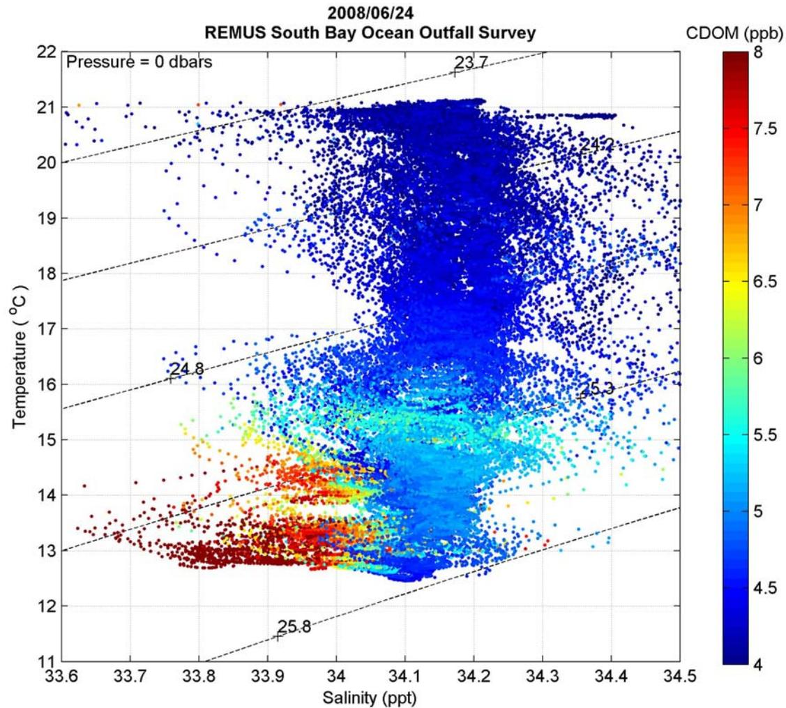
Temperature-Salinity (TS) diagram showing the distribution of watermasses by density (diagonal grid, units of  $\text{kg/m}^3 - 1000$ ) and CDOM concentration. The outfall plume is distinguished as a fresher (lower salinity) watermass with high CDOM concentrations ( $> 7$  ppb).
