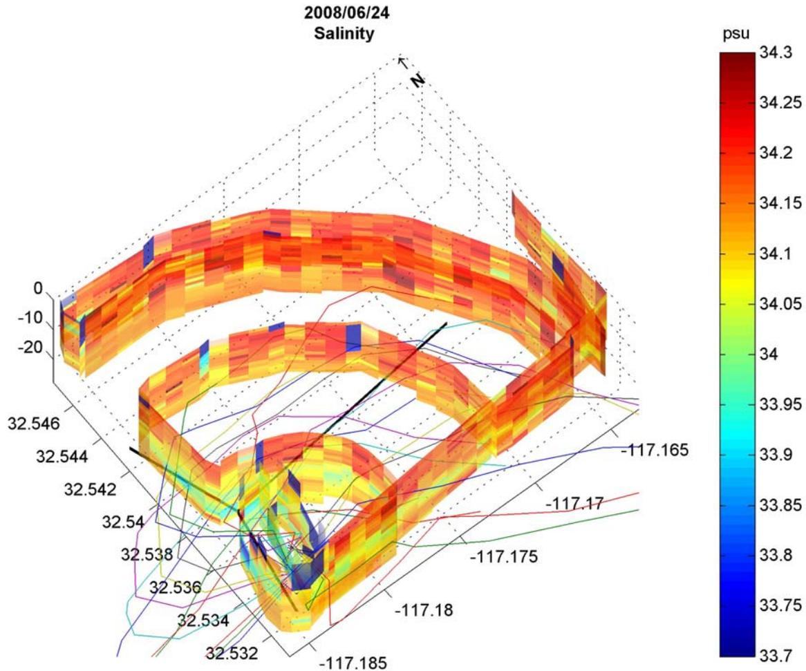
Salinity measurements shown with estimated SBOO plume trajectory (colored lines) based on near-realtime velocity profiles measured by the SBOO buoy. Low salinity near the outfall and eastward shows good agreement with the estimated trajectory.
