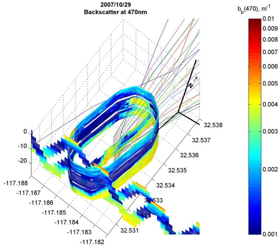
Near-field backscatter measurements at 470nm show good correspondence between elevated values ( $>0.003 m^{-1}$ ) and the estimated plume trajectory indicating elevated turbidity associated with the effluent.
