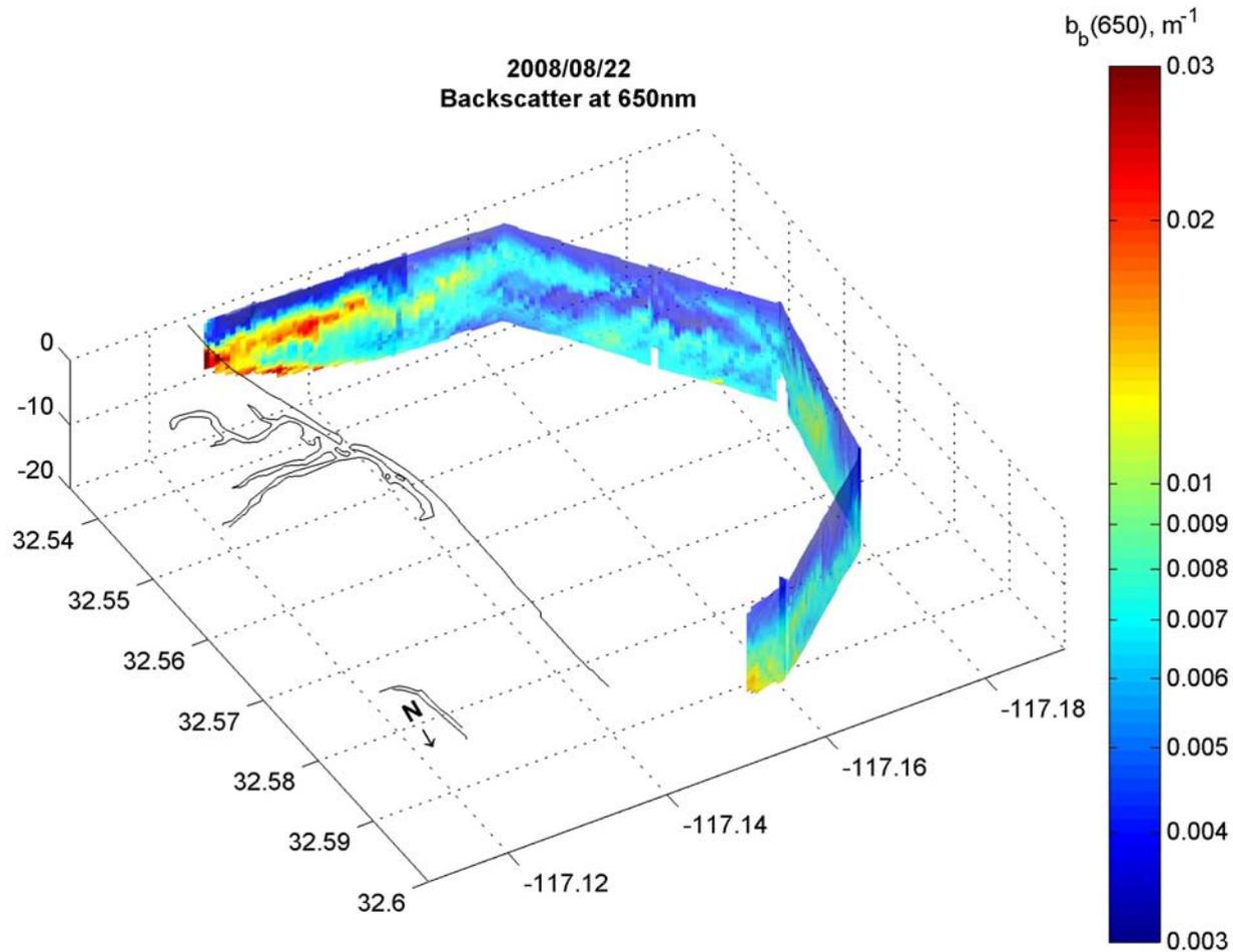
Backscatter measurements at 650 nm shows elevated values ( $>0.006 \text{ m}^{-1}$ ) near the seafloor and just below the thermocline. Possible sources of elevated backscatter include sediment resuspension and phytoplankton.
