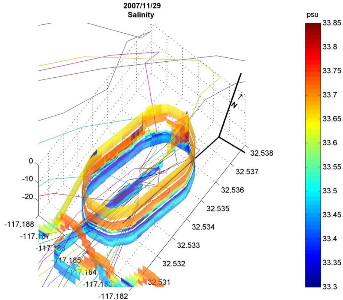
Salinity measurements shown with estimated SBOO plume trajectory (colored lines) based on near-realtime velocity profiles measured by the SBOO buoy. Low salinity at depth indicates the distribution of the SBOO plume.
