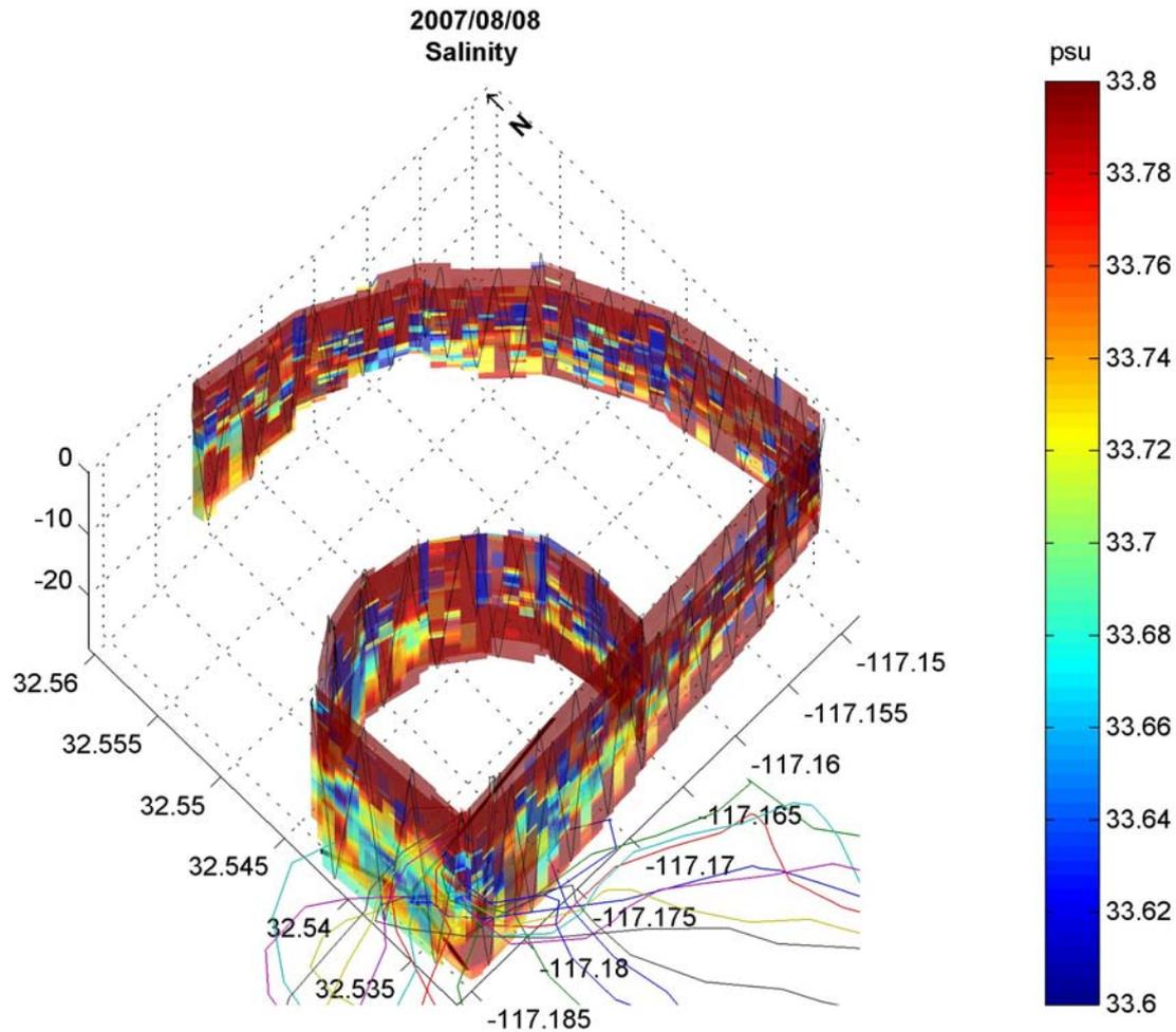
Salinity measurements shown with estimated SBOO plume trajectory (colored lines) based on near-realtime velocity profiles measured by the SBOO buoy. Noise at approximately 10m is due to transit across the thermocline. Low salinity (< 33.72 psu) near the outfall and around estimated trajectories indicate detection of the SBOO plume.
