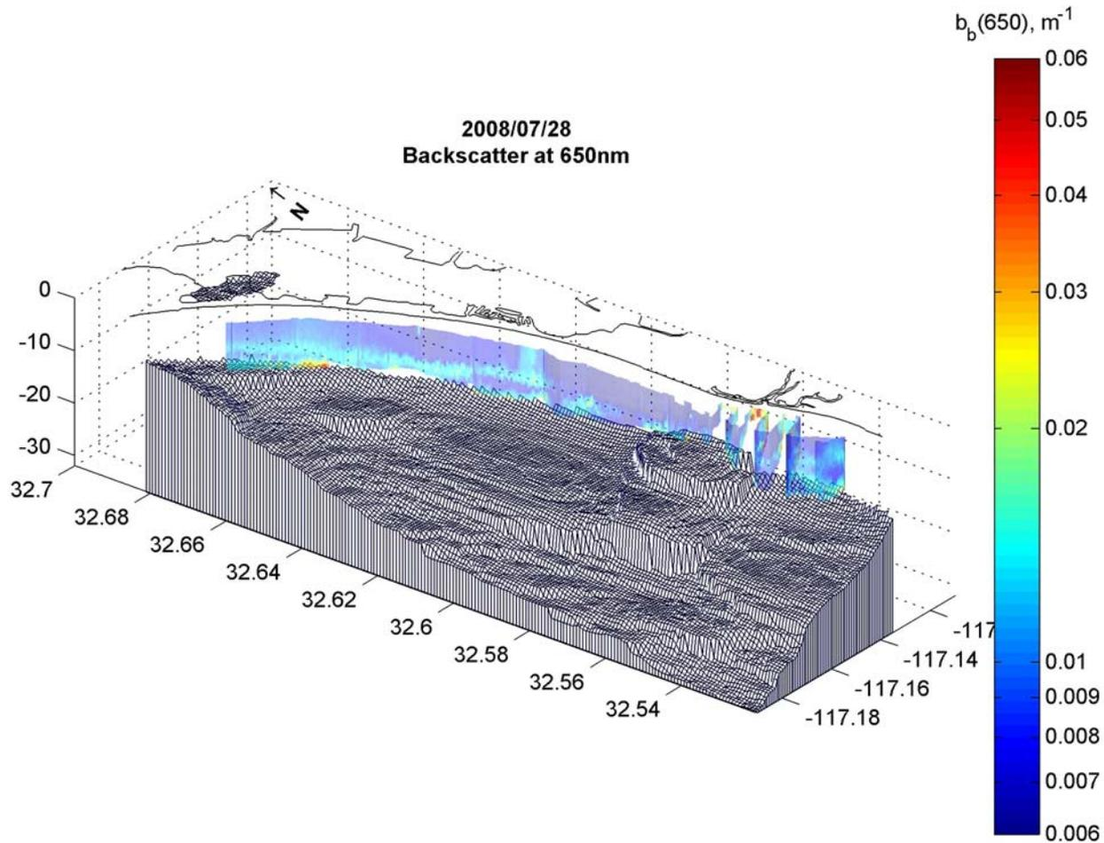
Backscatter measurements at 650 nm shows elevated values ( $>0.02 \text{ m}^{-1}$ ) near the surface at the Tijuana River mouth indicating exchange with the estuary during periods of no flow. Elevated values ( $>0.01 \text{ m}^{-1}$ ) near the seafloor may be due to sediment resuspension by currents scouring bottom sediment.
