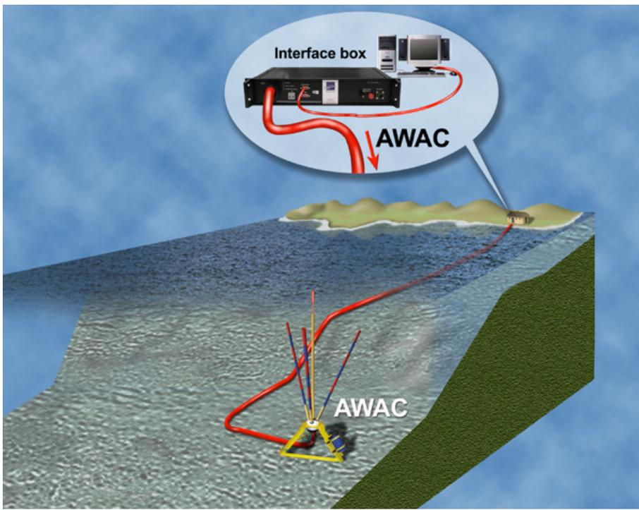
**Figure 13.** A concept drawing of the acoustic current meter / directional wave gauge that will be deployed from the Imperial Beach pier.
