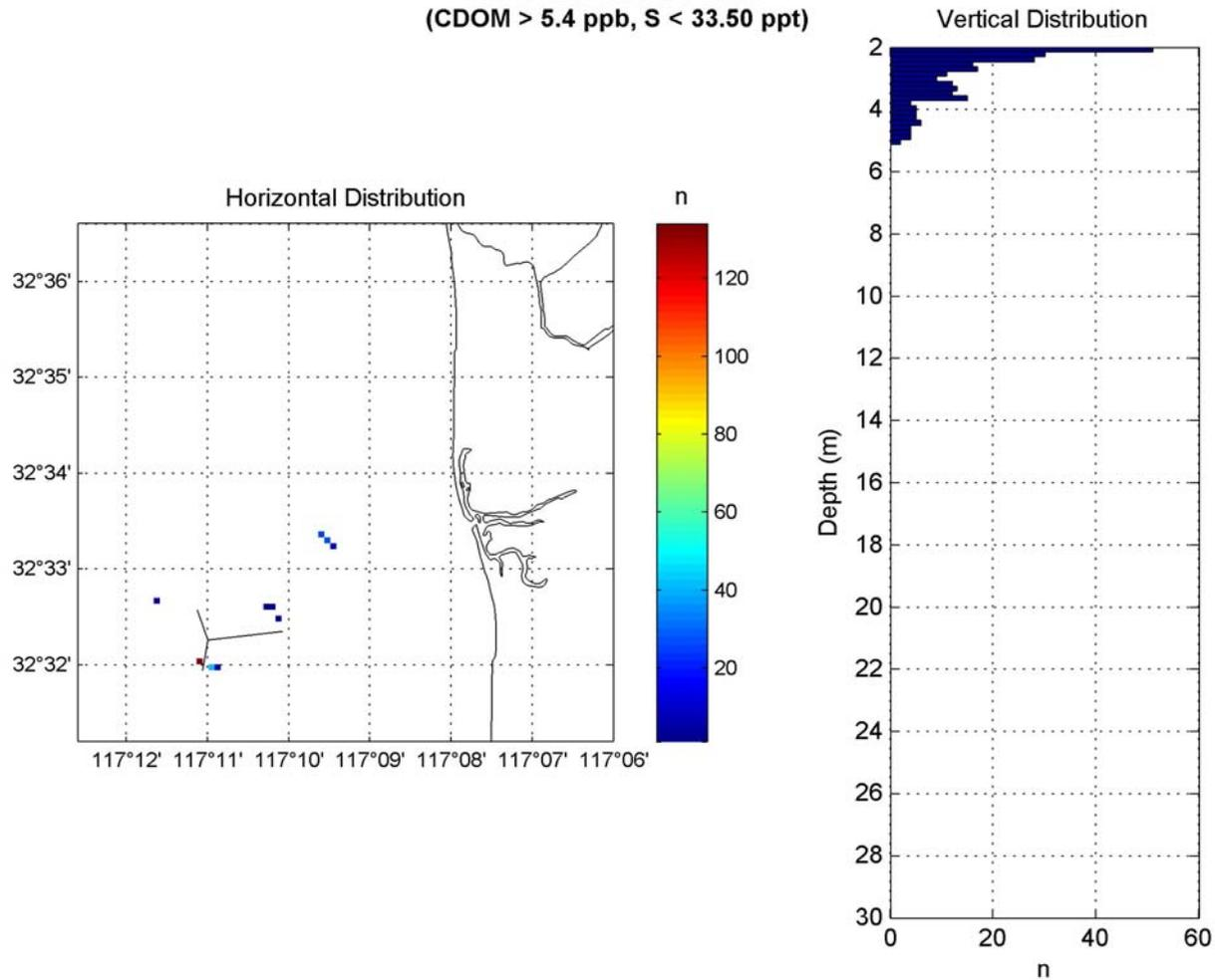
Horizontal and vertical plume distributions based on thresholding by the plumes' signature CDOM and salinity values. The number of samples satisfying the threshold criteria for a given horizontal or vertical bin is given by 'n'.
