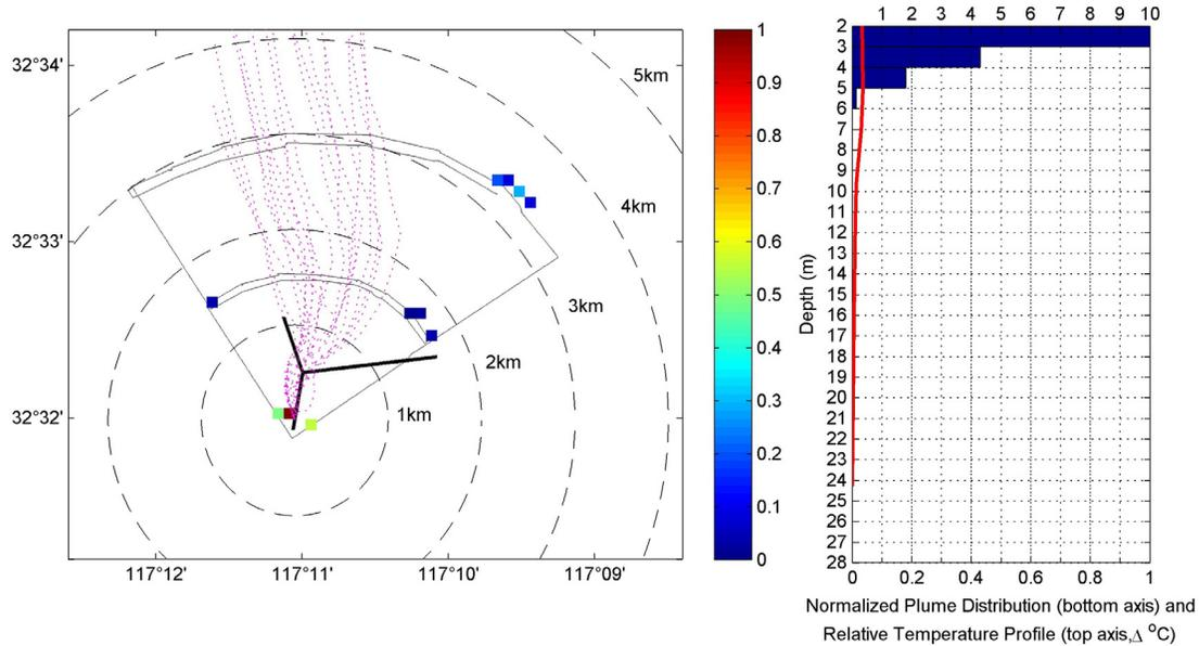
**Figure A.12 Horizontal and Vertical SBOO Plume Trajectory – February 15, 2008**
