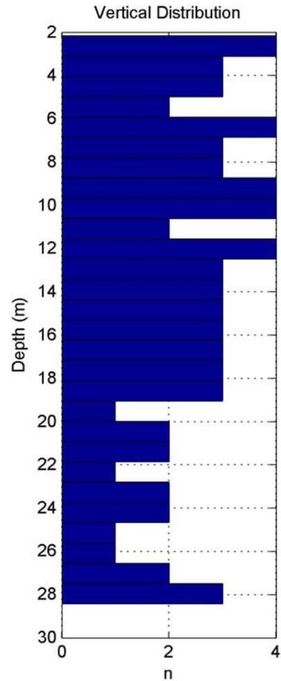
Horizontal and vertical plume distributions based on thresholding by the plumes' signature salinity value. The number of samples satisfying the threshold criteria for a given horizontal or vertical bin is given by 'n'.
