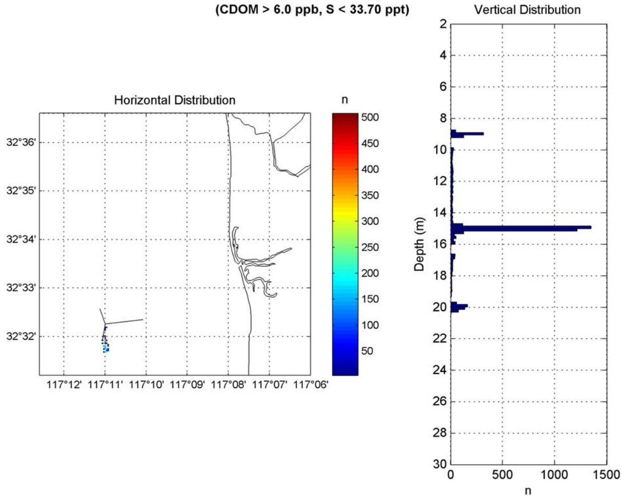
Horizontal and vertical plume distributions based on thresholding by the plumes' signature CDOM and salinity values. The number of samples satisfying the threshold criteria for a given horizontal or vertical bin is given by 'n'.
