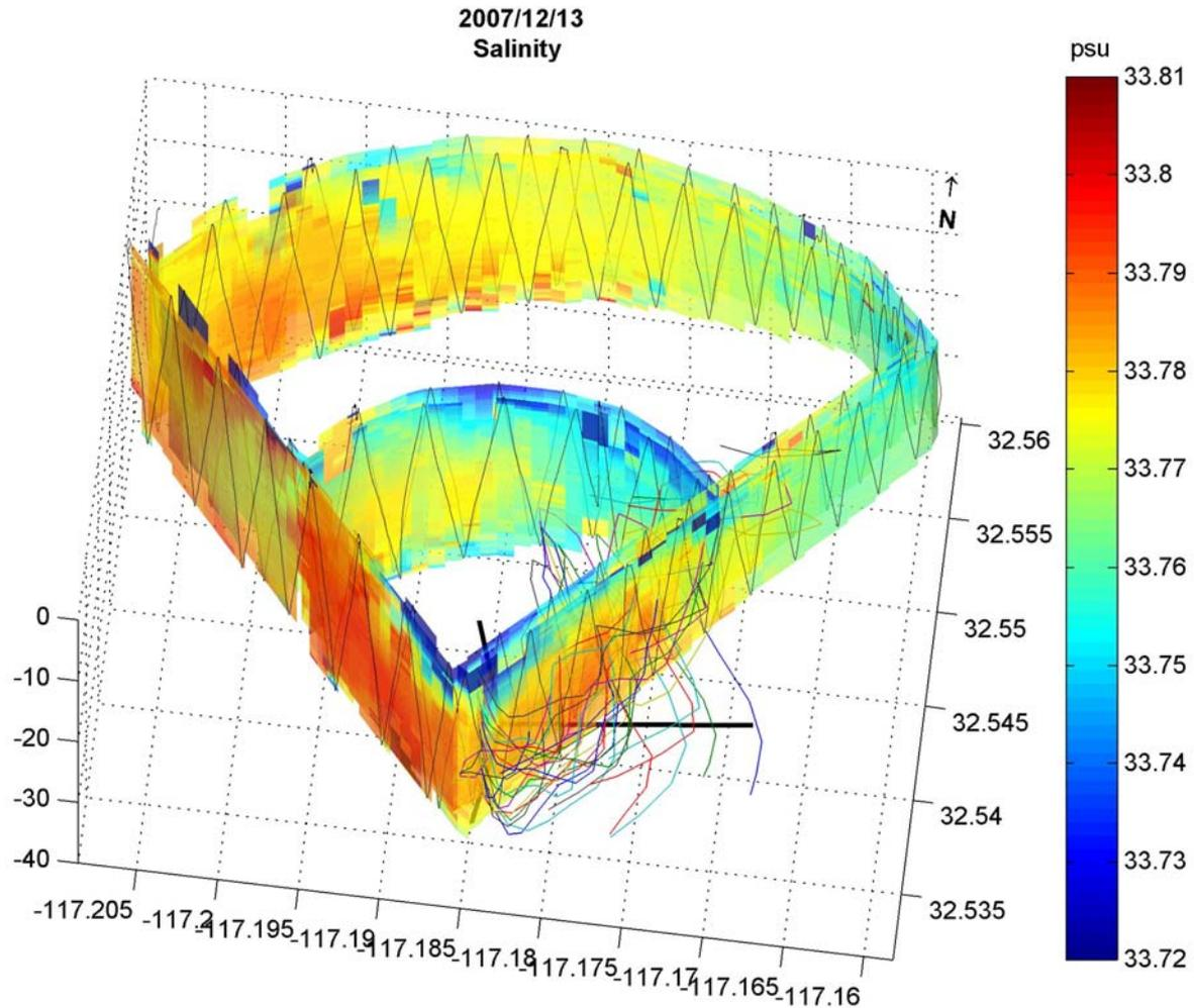
Salinity measurements shown with estimated SBOO plume trajectory (colored lines) based on near-realtime velocity profiles measured by the SBOO buoy. Low salinity near the outfall and northward following the estimated trajectory shows the SBOO plume rises quickly and surfacing.
