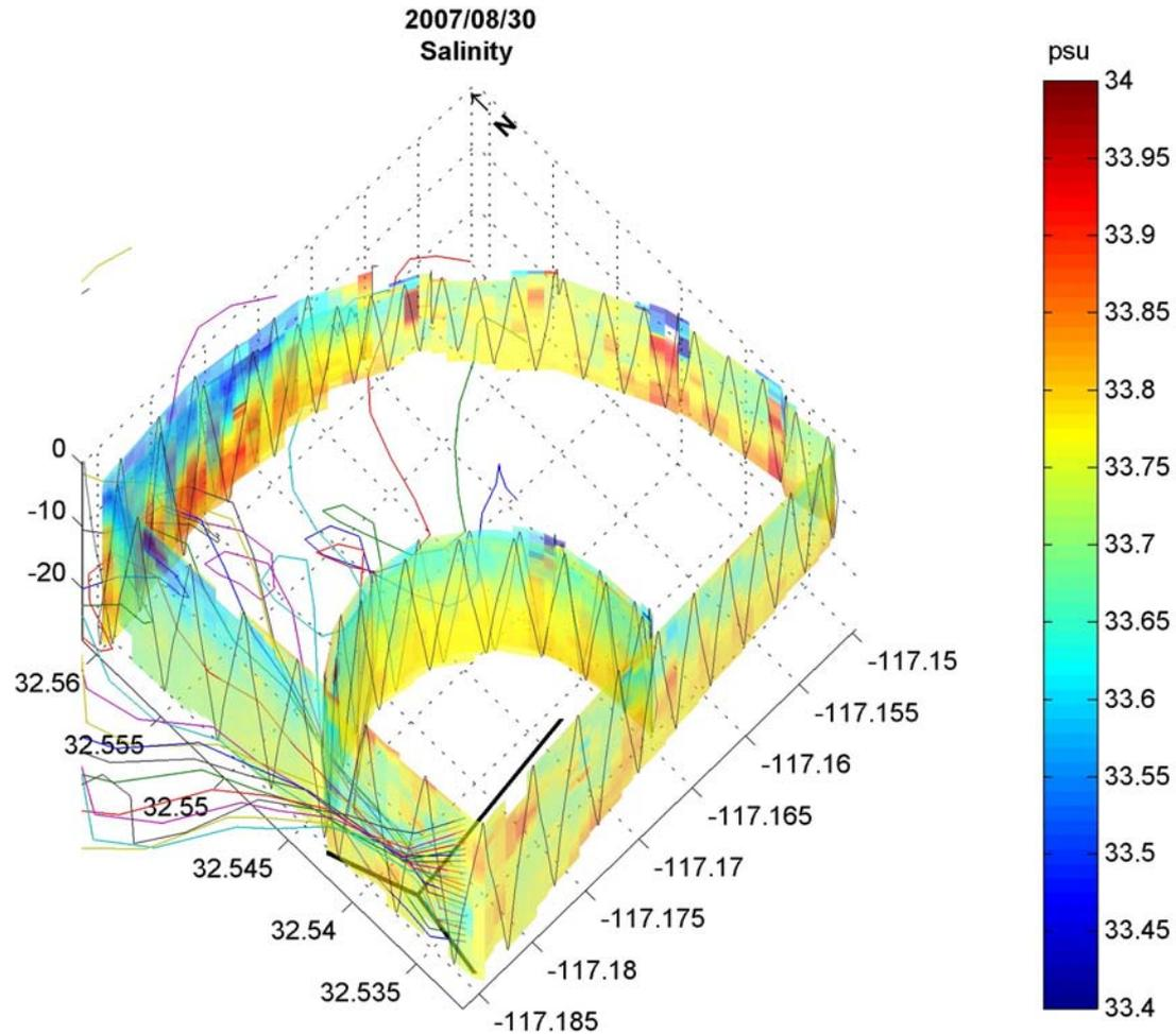
Salinity measurements shown with estimated SBOO plume trajectory (colored lines) based on near-realtime velocity profiles measured by the SBOO buoy. Low salinity near the outfall and northward shows the SBOO plume rising and surfacing.
