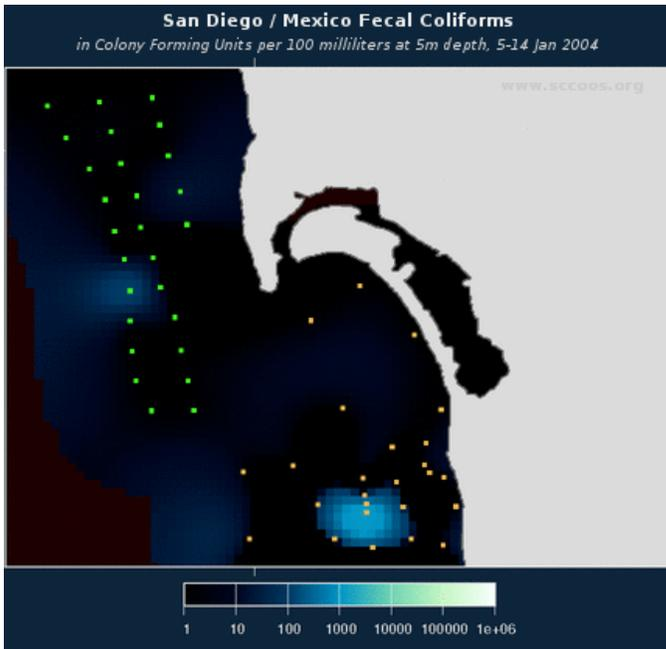
**Figure 5.** Spatial patterns of fecal coliform levels at 5m depth as measured by the existing SBOO permit activities. The data illustrates high levels of FIB near the SBOO outfall (top) and near the Tijuana River (bottom).
