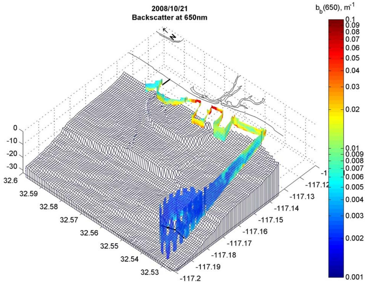
Backscatter measurements at 650 nm shows elevated values ( $>0.02 m^{-1}$ ) near the Tijuana River mouth indicating exchange with the estuary during periods of no flow.
