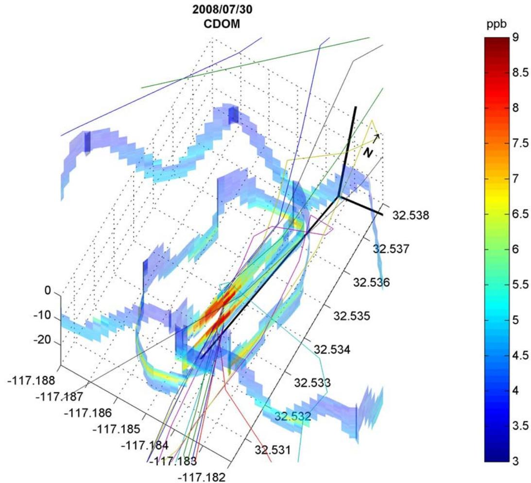
Near-field CDOM measurements greater than 5.5 ppb show good correspondence with the estimated SBOO plume trajectory (colored lines) based on near-real-time velocity profiles measured by the SBOO buoy.
