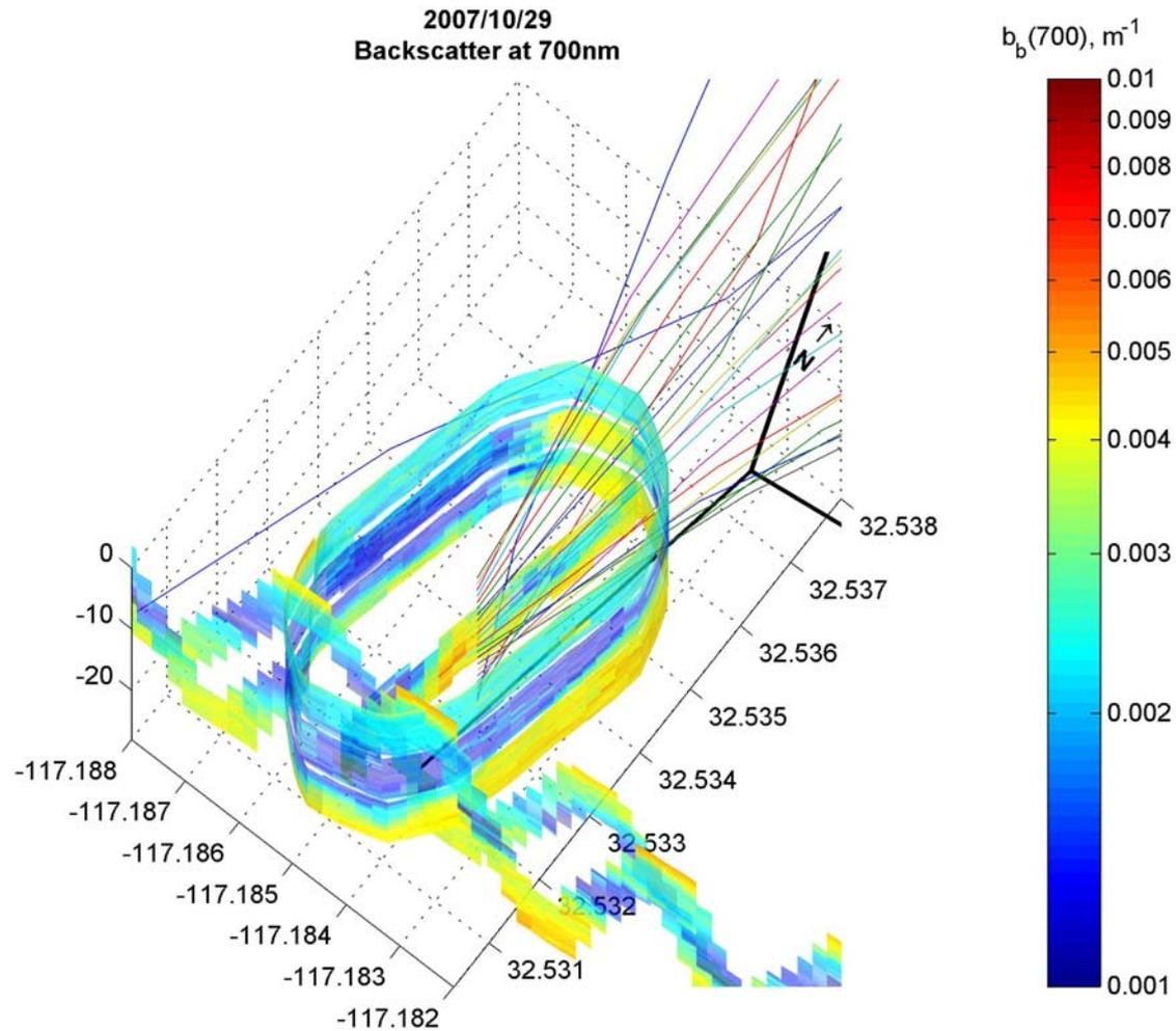
Near-field backscatter measurements at 700nm show good correspondence between elevated values ( $>0.004 \text{ m}^{-1}$ ) and the estimated plume trajectory indicating elevated turbidity associated with the effluent.
