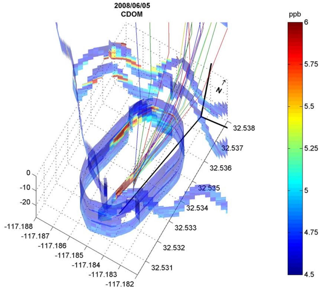
Near-field CDOM measurements greater than 5 ppb show good correspondence with the estimated SBOO plume trajectory (colored lines) based on near-realtime velocity profiles measured by the SBOO buoy.
