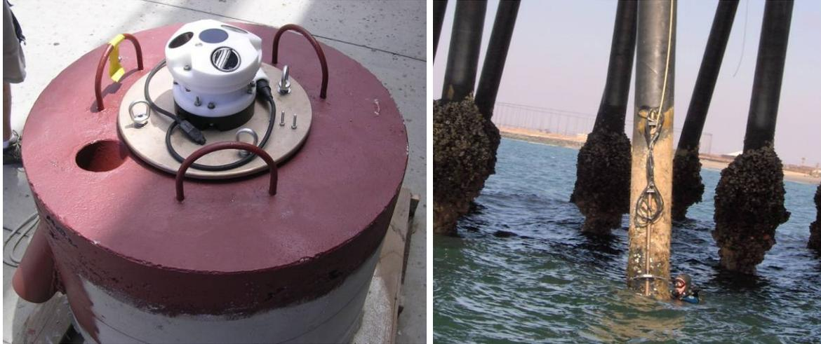
**Figure D.4 Acoustic Wave and Current Profiler**
