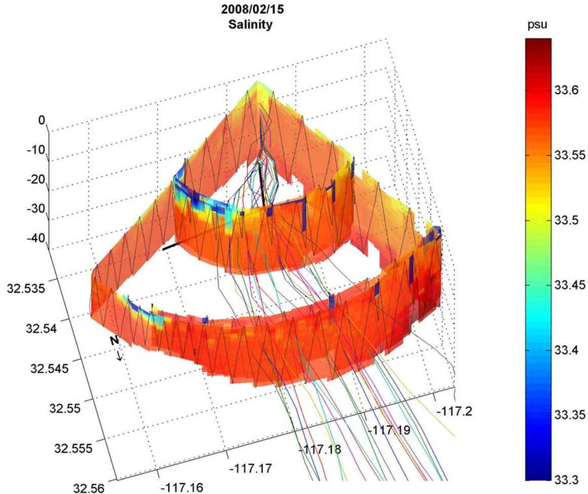
Salinity measurements shown with estimated SBOO plume trajectory (colored lines) based on near-realtime velocity profiles measured by the SBOO buoy. Low salinity near the outfall and northward following the estimated trajectory shows the SBOO plume rose quickly and surfaced.
