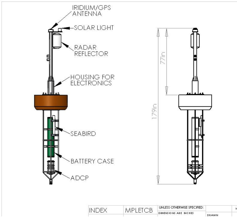
**Figure 10.** Mechanical drawing of the surface buoy to be deployed near the WYE of the SBOO. Not shown is the temperature chain which will measure ocean temperatures from 1m to the seafloor at approximately 3m spacing.
