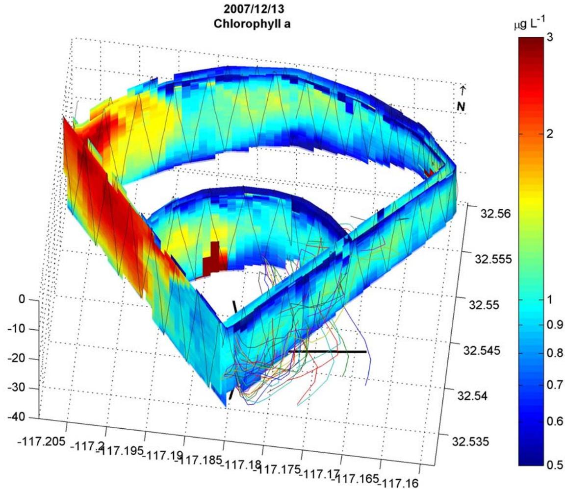
Chlorophyll a measurements shown with estimated SBOO plume trajectory (colored lines) based on near-realtime velocity profiles measured by the SBOO buoy. Correspondence between salinity and the estimated plume trajectory suggests that the SBOO plume is low in chlorophyll a ( $<0.7 \mu\text{g L}^{-1}$ ).
