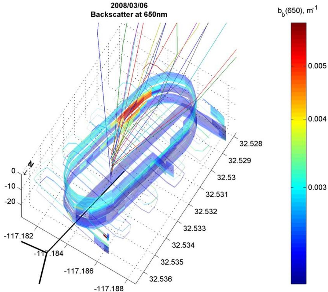
Near-field backscatter measurements at 650 nm shows good correspondence between elevated values ( $>0.004 m^{-1}$ ) and the estimated plume trajectory indicating elevated turbidity associated with the effluent.
