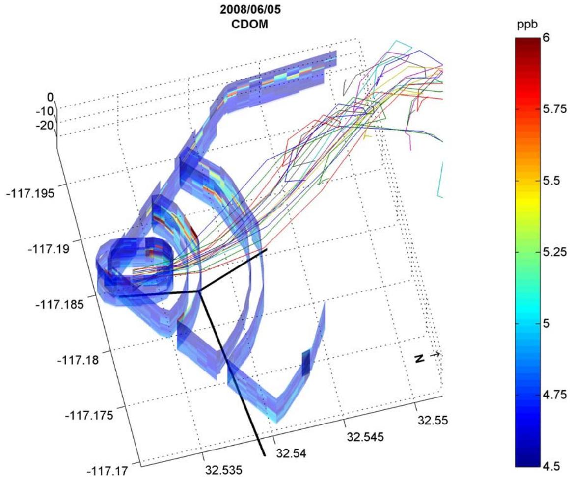
Elevated CDOM measurements (> 5 ppb) show good correspondence with estimated SBOO plume trajectory (colored lines) based on near-realtime velocity profiles measured by the SBOO buoy.
