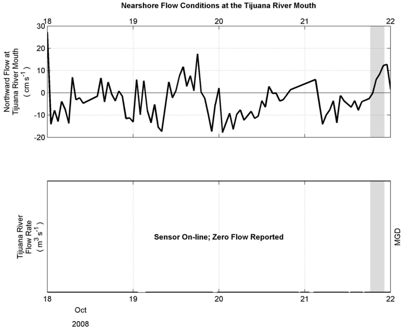
Alongshore surface current velocity measured by HF-Radar at the Tijuana River mouth (top) and flow rate from the Tijuana River as measured by the IBWC gauge (bottom). The grey panel indicates the sampling period.
