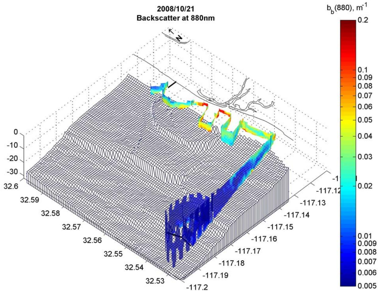
Backscatter measurements at 880 nm shows elevated values ( $>0.05 m^{-1}$ ) near the Tijuana River mouth indicating exchange with the estuary during periods of no flow.
