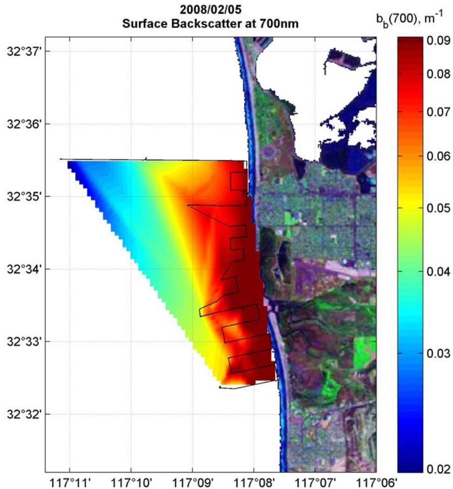
Elevated ( $>0.03 m^{-1}$ ) nearshore surface backscatter measurements at 700 nm indicate elevated turbidity associated the Tijuana River plume.
