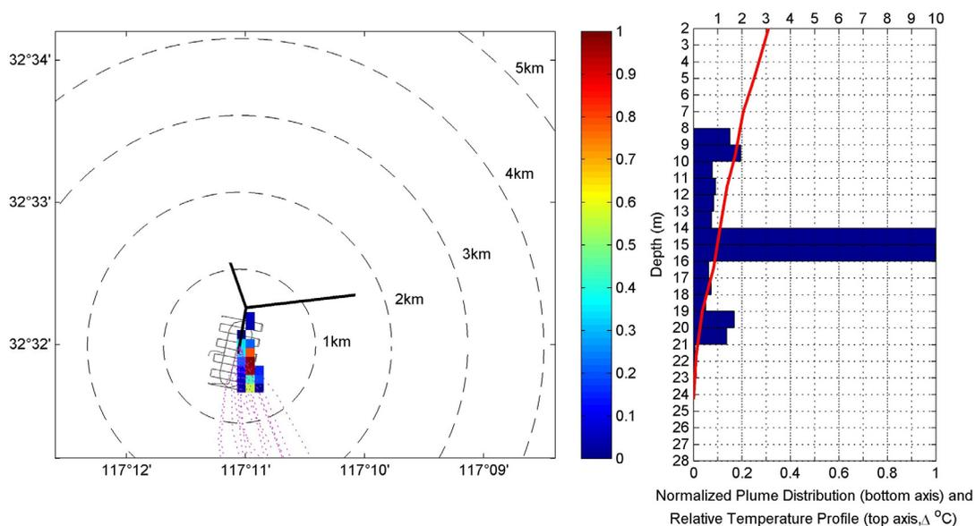
**Figure A.8 Horizontal and Vertical SBOO Plume Distributions – March 6, 2008**
