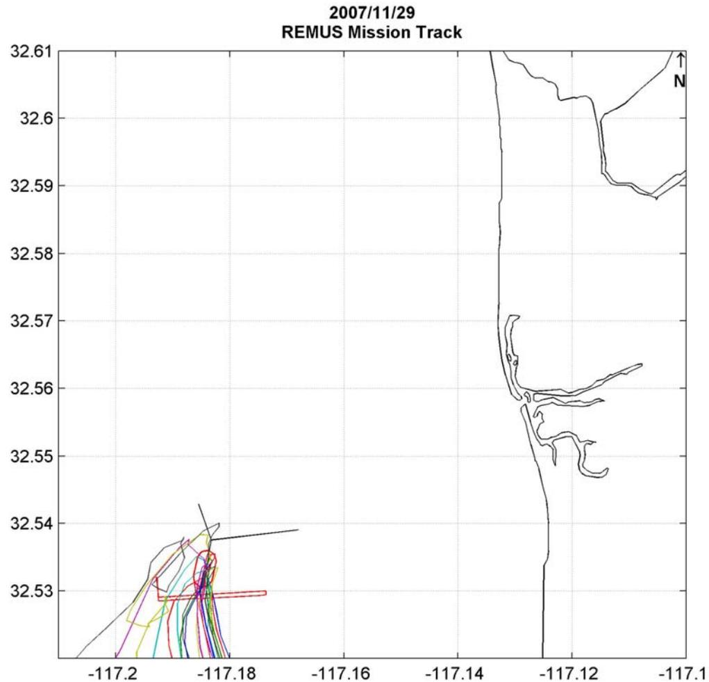
REMUS Mission track (red) and estimated SBOO plume trajectory (colored lines) based on near-realtime velocity profiles measured by the SBOO buoy.
