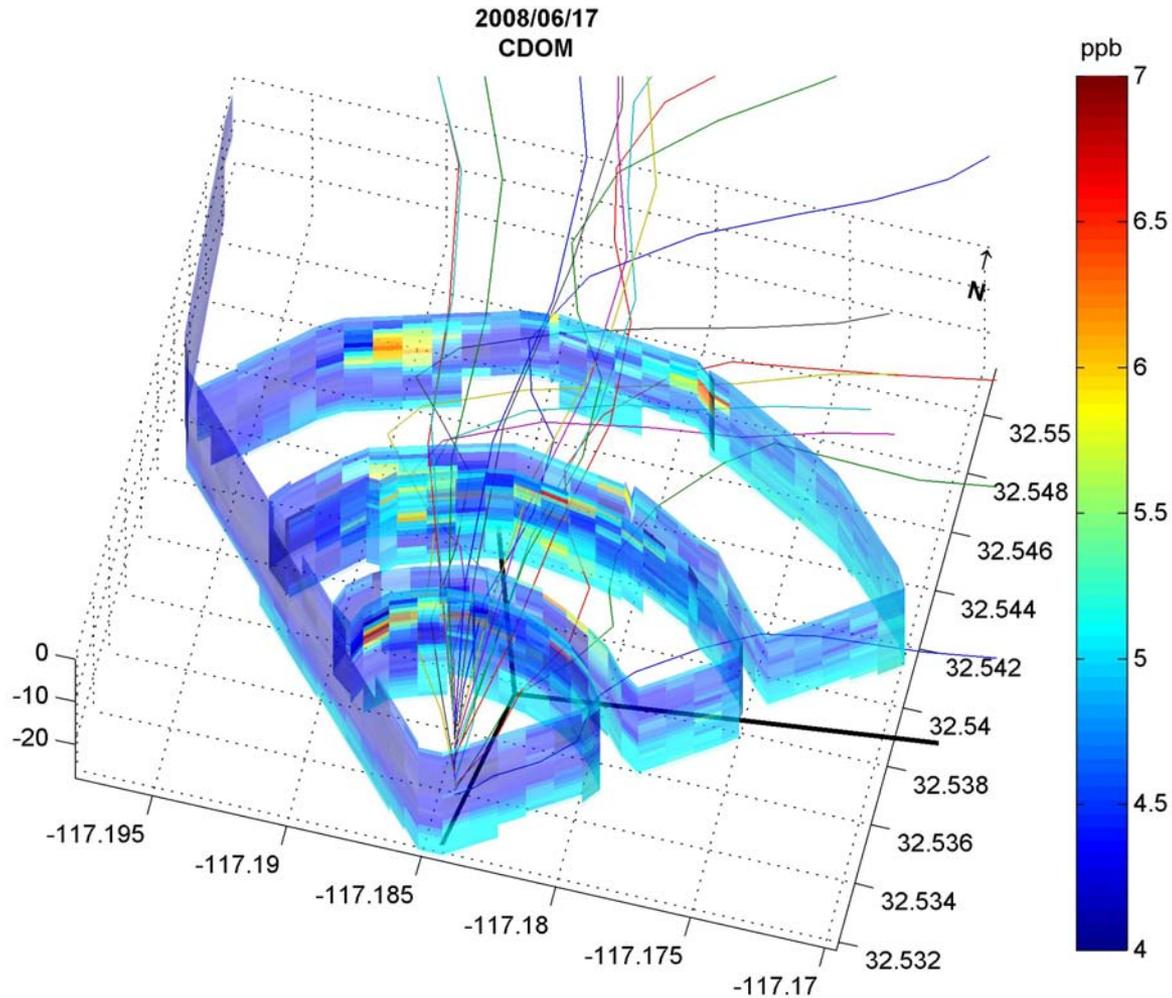
Elevated CDOM measurements ( $> 5$  ppb) show good correspondence with the estimated SBOO plume trajectory (colored lines) based on near-realtime velocity profiles measured by the SBOO buoy.
