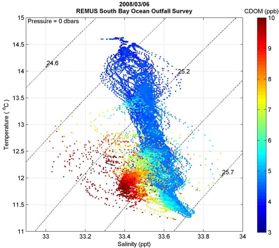
Temperature-Salinity (TS) diagram showing the distribution of watermasses by density (diagonal grid, units of  $\text{kg/m}^3 - 1000$ ) and CDOM concentration. The outfall plume is distinguished as a fresher (lower salinity) watermass with high CDOM concentrations ( $> 6$  ppb).
