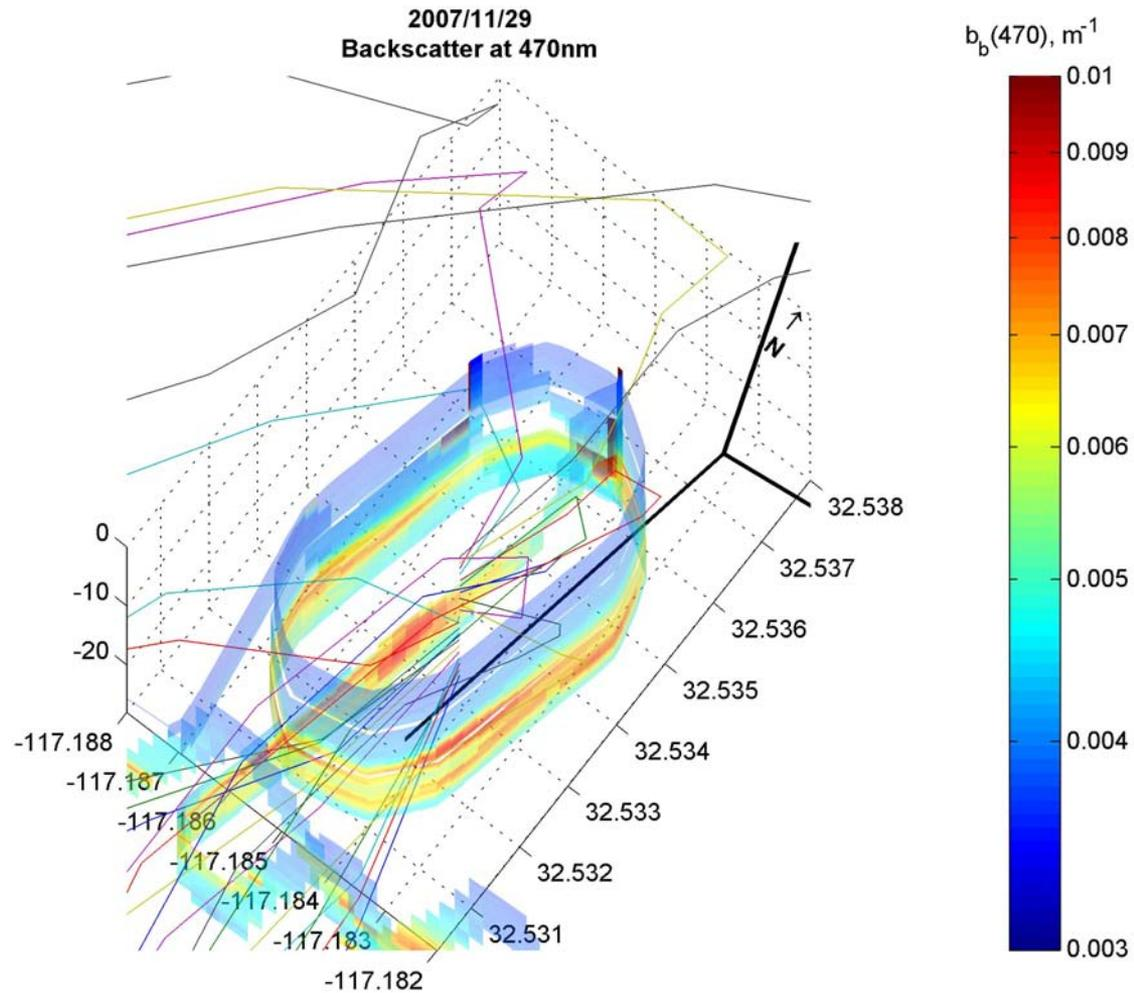
Near-field backscatter measurements at 470nm show good correspondence between elevated values ( $>0.006 \text{ m}^{-1}$ ) and the estimated plume trajectory indicating elevated turbidity associated with the effluent.
