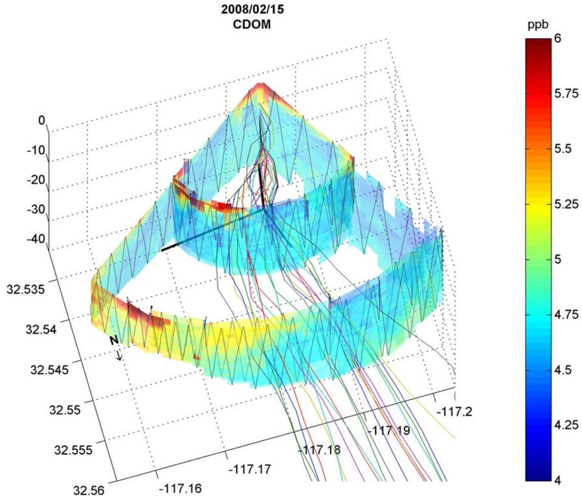
CDOM measurements shown with estimated SBOO plume trajectory (colored lines) based on near-realtime velocity profiles measured by the SBOO buoy. Elevated CDOM (> 5 ppb) near the outfall and northward following the estimated trajectory shows the SBOO plume rose quickly and surfaced.
