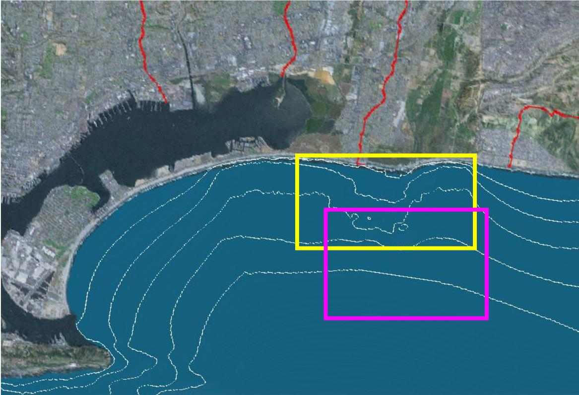
**Figure 3.** General region of survey interest for mapping the SBOO (purple) and Tijuana River plume (yellow). Depth contours shown at 5m, 10m, 15m, 20m, and 25m. Surveys for the Tijuana River plume will nominally extend from the 5m to 20m isobaths while the SBOO plume surveys will be focused in the region of the outfall. While not represented by the purple box, the program will support tracking to its furthest, detectable extent.
