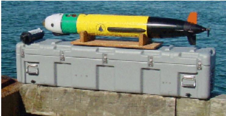
**Figure 2.** The REMUS autonomous underwater vehicle. A vehicle equipped with sensors specific for tracking the plumes of the Tijuana River and South Bay Ocean Outfall will be routinely deployed in support of this program.
