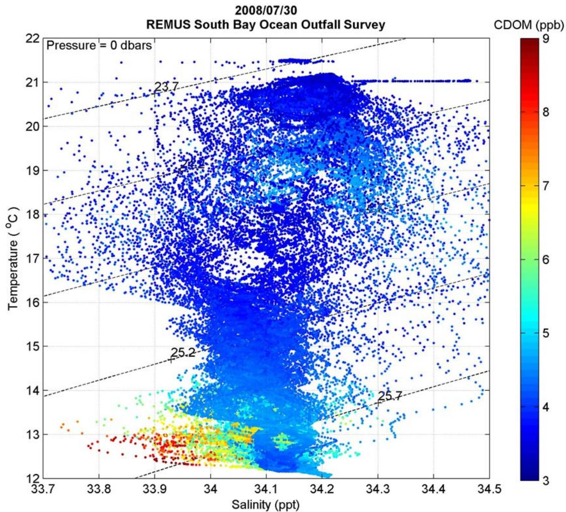
Temperature-Salinity (TS) diagram showing the distribution of watermasses by density (diagonal grid, units of  $\text{kg/m}^3 - 1000$ ) and CDOM concentration. The outfall plume is distinguished as a fresher (lower salinity) watermass with high CDOM concentrations ( $> 5.5$  ppb).
