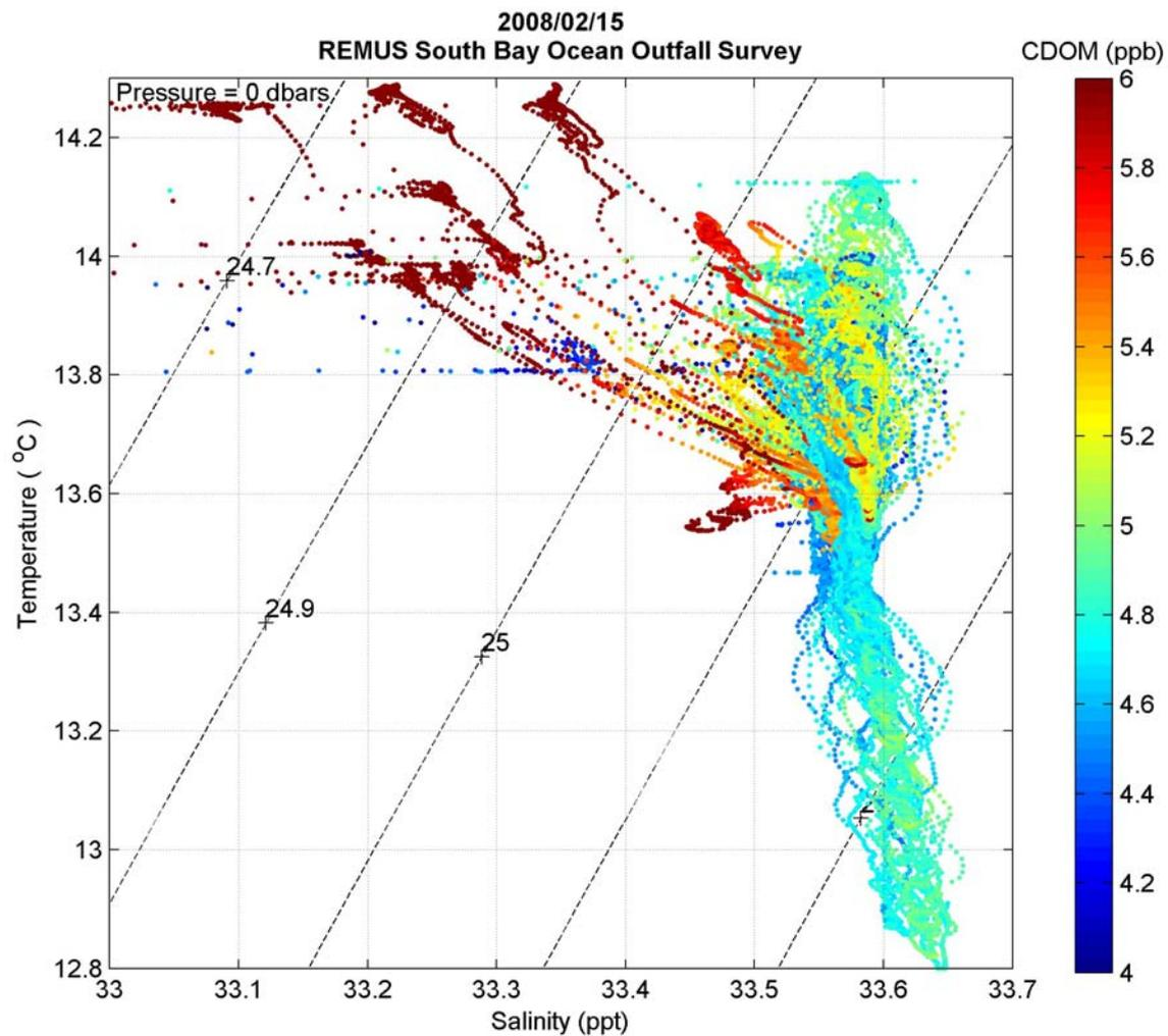
Temperature-Salinity (TS) diagram showing the distribution of watermasses by density (diagonal grid, units of  $\text{kg/m}^3 - 1000$ ) and CDOM concentration. The outfall plume is distinguished as a fresher (lower salinity) watermass with high CDOM concentrations ( $> 5.4$  ppb).
