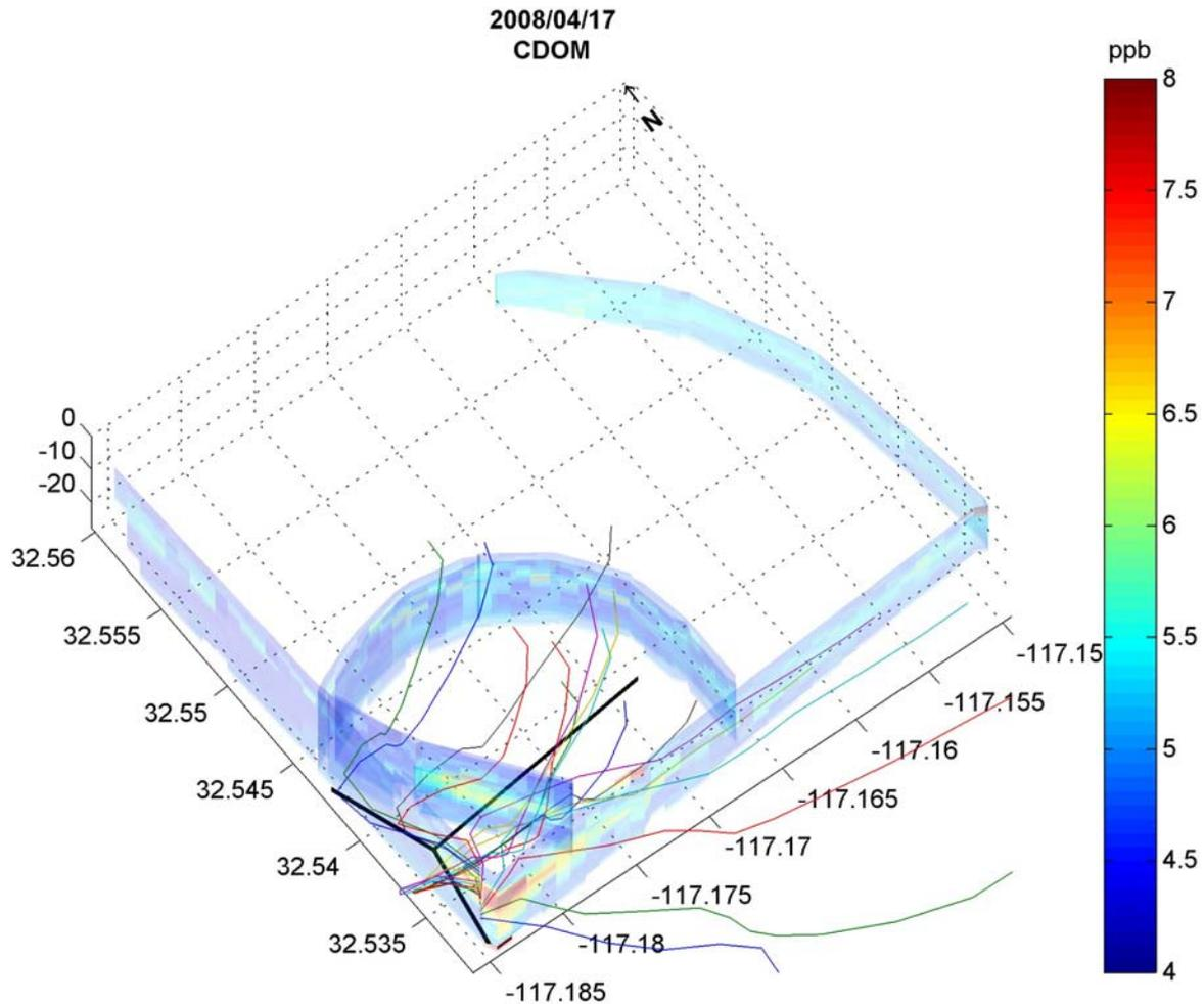
Correspondence between elevated CDOM measurements in the southwest over the outfall and estimated SBOO plume trajectory (colored lines) based on near-realtime velocity profiles measured by the SBOO buoy.
