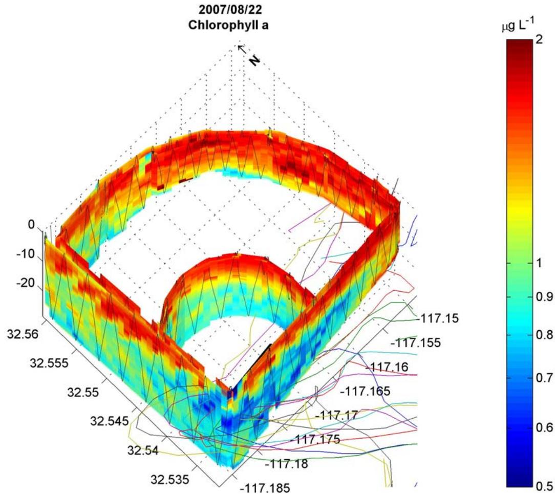
Chlorophyll a measurements shown with estimated SBOO plume trajectory (colored lines) based on near-realtime velocity profiles measured by the SBOO buoy. Correspondence between salinity and the estimated plume trajectory suggests that the SBOO plume is low in chlorophyll a ( $<0.7 \mu\text{g L}^{-1}$ ).
