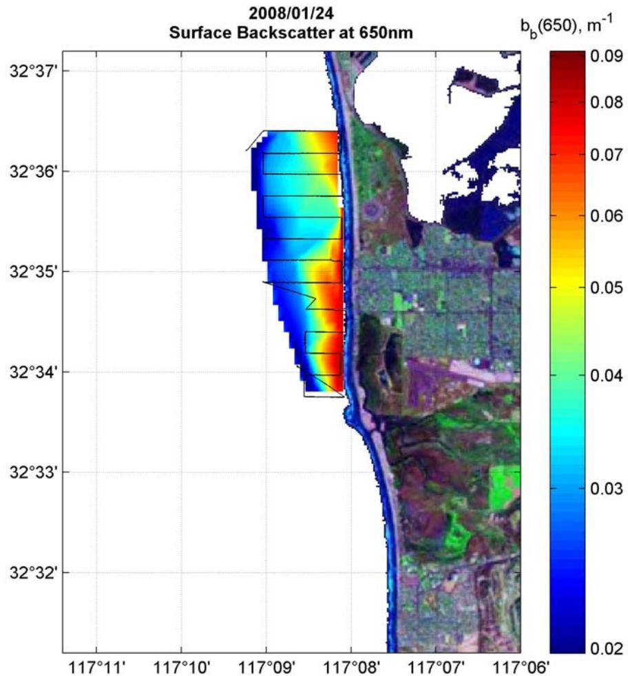
Elevated ( $>0.03 m^{-1}$ ) nearshore surface backscatter measurements at 650nm indicate elevated turbidity associated the Tijuana River plume.
