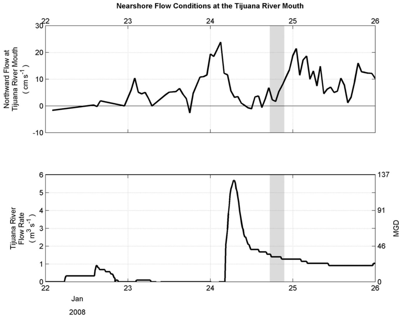
Alongshore surface current velocity measured by HF-Radar at the Tijuana River mouth (top) and flow rate from the Tijuana River as measured by the IBWC gauge (bottom). The grey panel indicates the sampling period.
