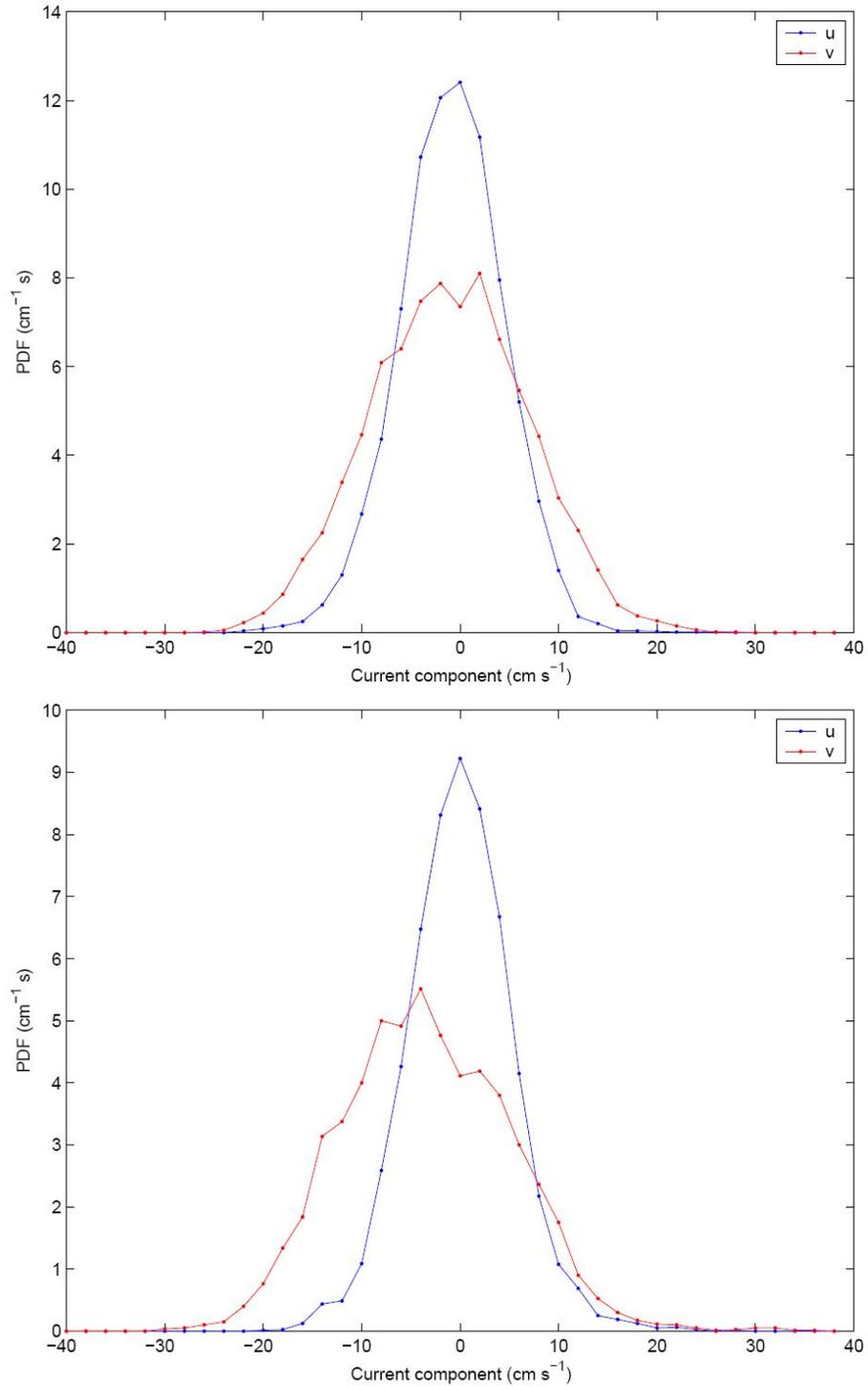
**Figure D.10 Depth-Averaged Currents Probability Distribution**
