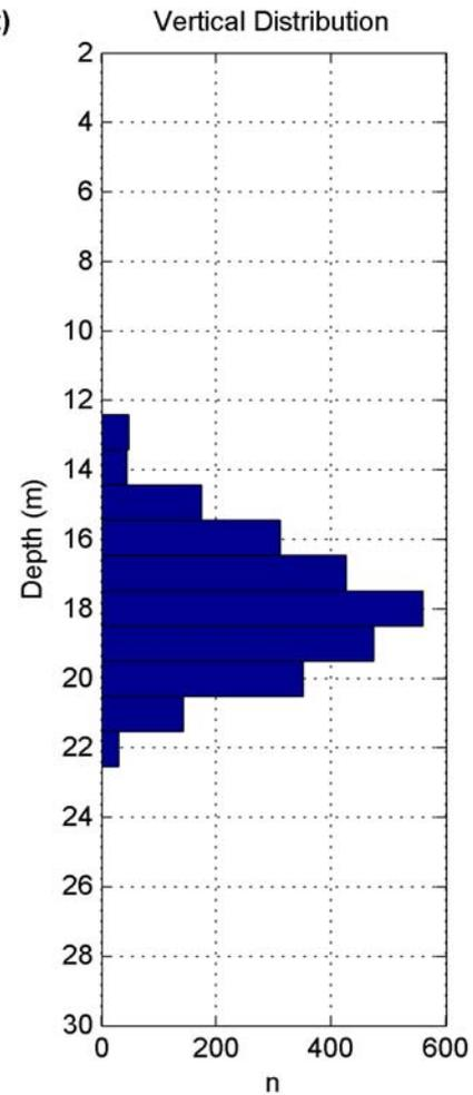
Horizontal and vertical plume distributions based on thresholding by the plumes' signature CDOM and salinity values. The number of samples satisfying the threshold criteria for a given horizontal or vertical bin is given by 'n'.
