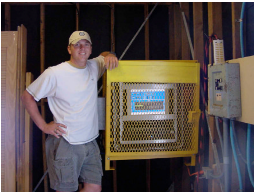
Figure 6. The data and power cable are connected to the computer logging system that is located on the bottom floor of the lifeguard tower.
