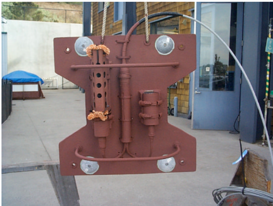
Figure 4. The sensor system ready to be deployed. Here the mounts have also been painted with anti-fouling paint. The copper 'brillo' pads are fixed to either end of the conductivity and temperature probe to provide additional anti-fouling protection. Also shown is the armored cable that provides power and communication to the system.
