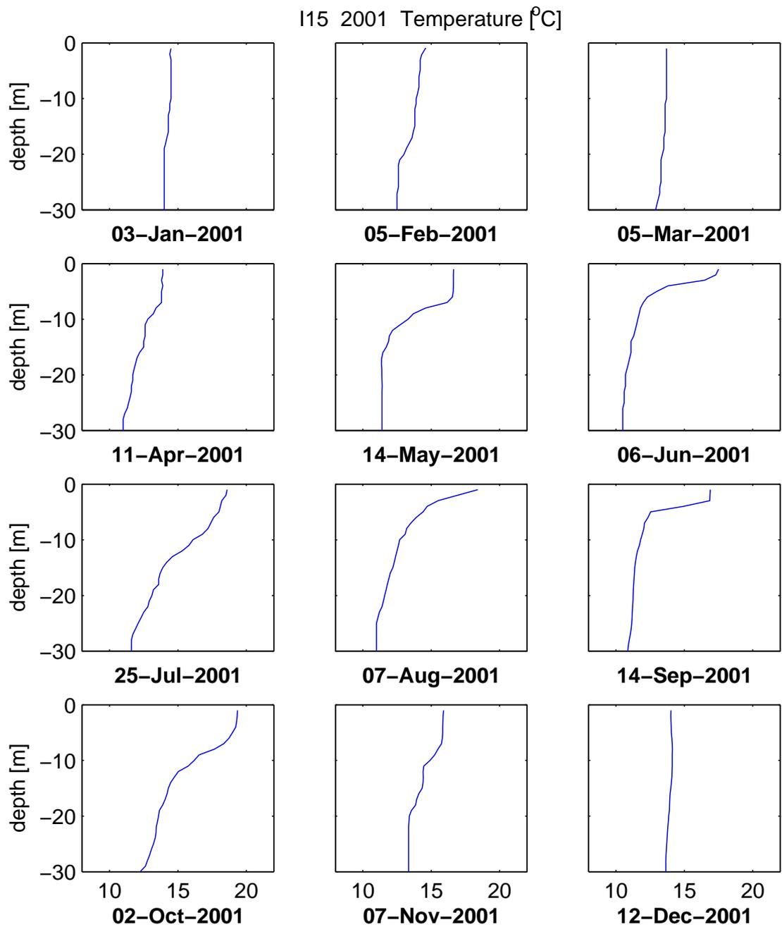
Figure 4.9: Temperature profiles from monthly ocean monitoring CTD surveys, 2001, at station I15 just offshore of the outfall wye.
