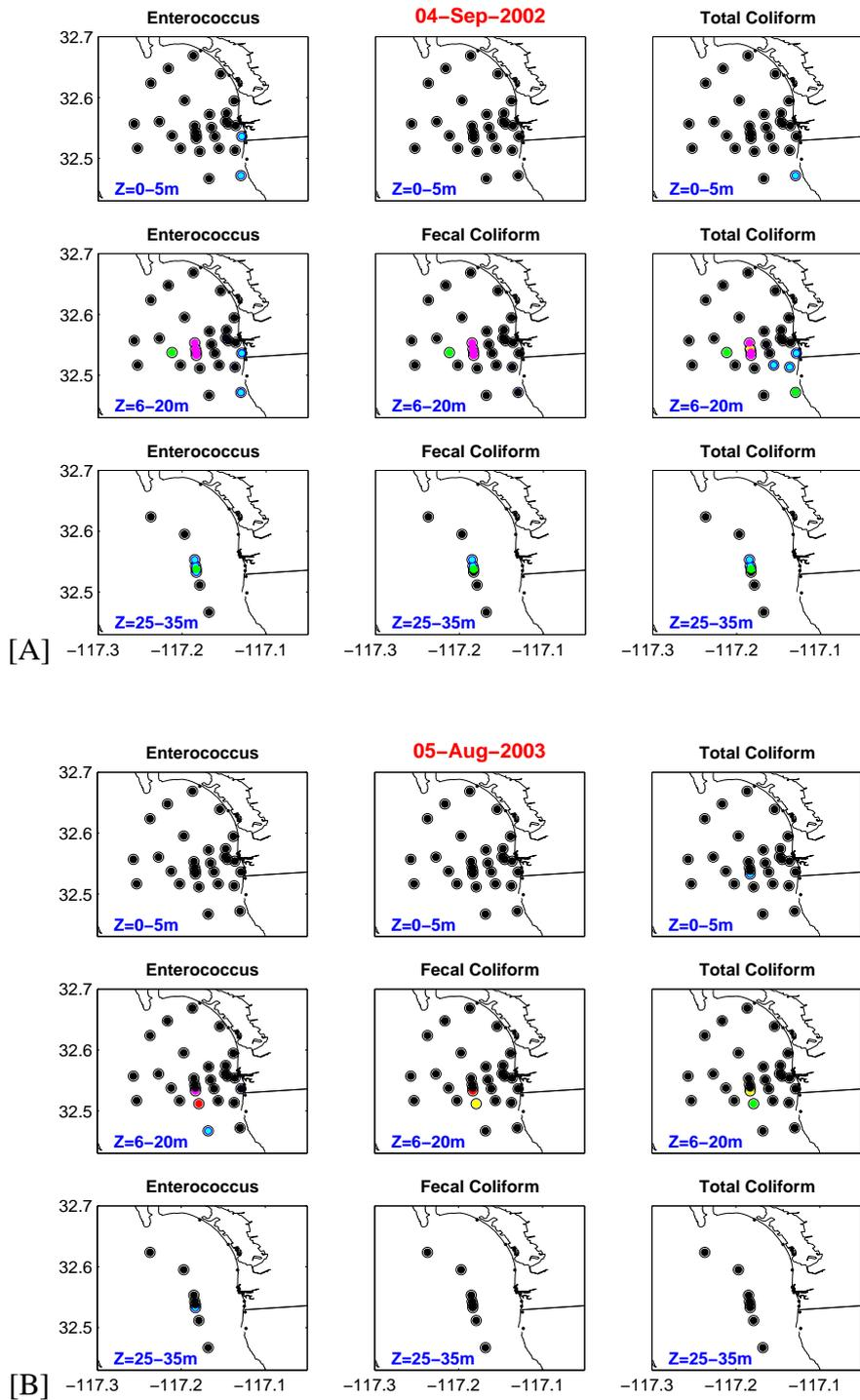
Figure 5.2: A) Bacterial sampling results for September 2002 CTD survey showing plume at mid-depth. B) August 2003 CTD survey showing plume at mid-depth travelling southward from the outfall. See color coding key in Table 5.1.
