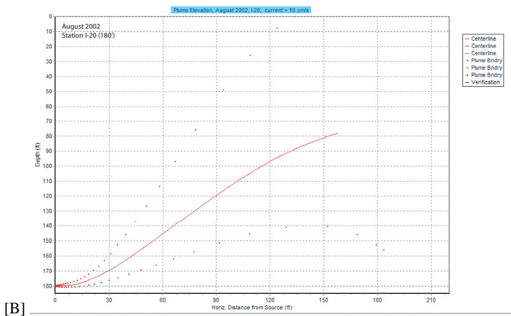
Figure 5.15: Predicted plume height during strong upwelling conditions: A) August 2001 CTD survey. Station I12 with 10 cm/s current velocity. B) August 2002 CTD survey, at deeper release site, Station I20 (180') with 10 cm/s current velocity.
