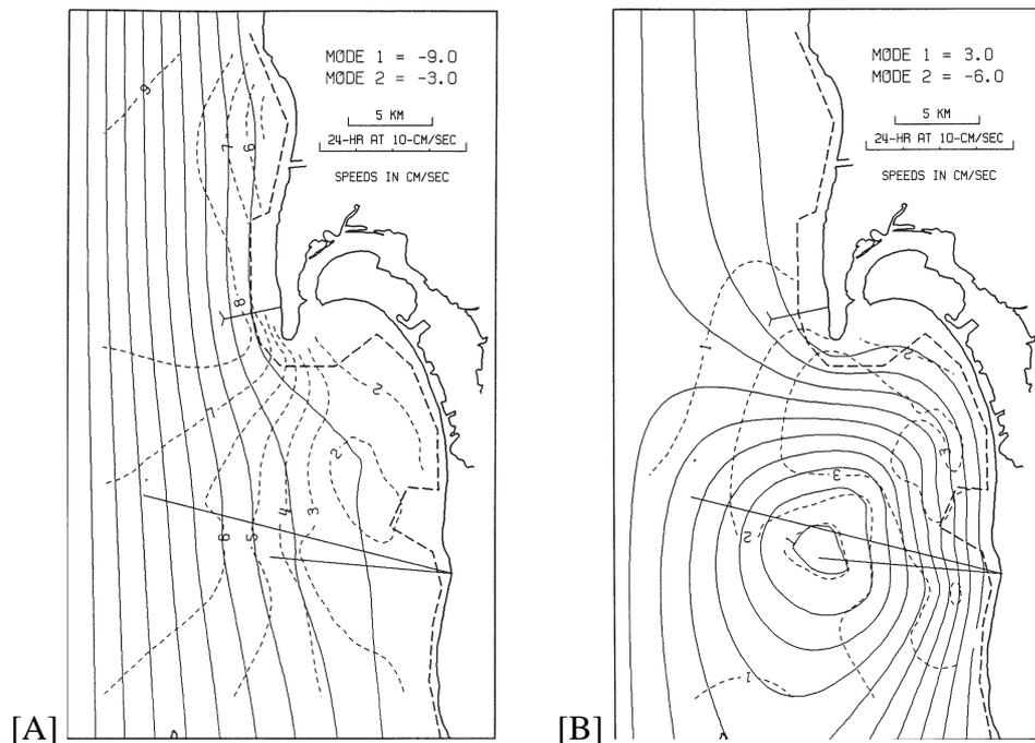
Figure 4.5: Composite model flows with highest probability of occurrence. A) Composite flow pattern with Mode 1 dominant. B) Composite flow pattern with Mode 2 dominant. The magnitude and direction of each mode is shown at the upper left (negative = down-coast/counterclockwise). Solid contours are streamlines, dashed are velocity contours. From *Hendricks & Christensen, 1987*.
