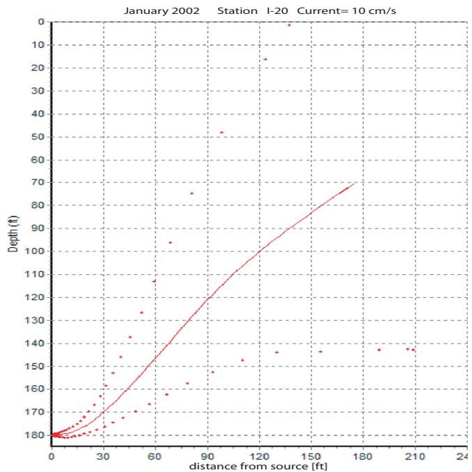
Figure 5.12: Predicted plume rise heights using CTD profiles from January 2002, Station I20, depth 180 ft. Solid red line is plume center, dotted line is boundary.
