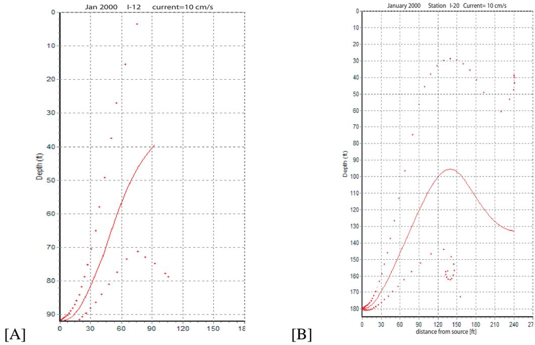
Figure 5.11: Predicted plume rise heights using CTD profiles from 3-5 January 2000, A) Station I12, near outfall. B) Station I20, depth 180 ft. Solid red line is plume center, dotted line is boundary.
