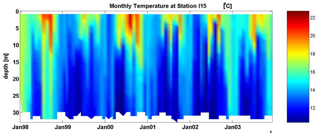
Figure 4.8: Water column temperature at CTD station I15, just offshore of outfall wye. January 1998-December 2003.
