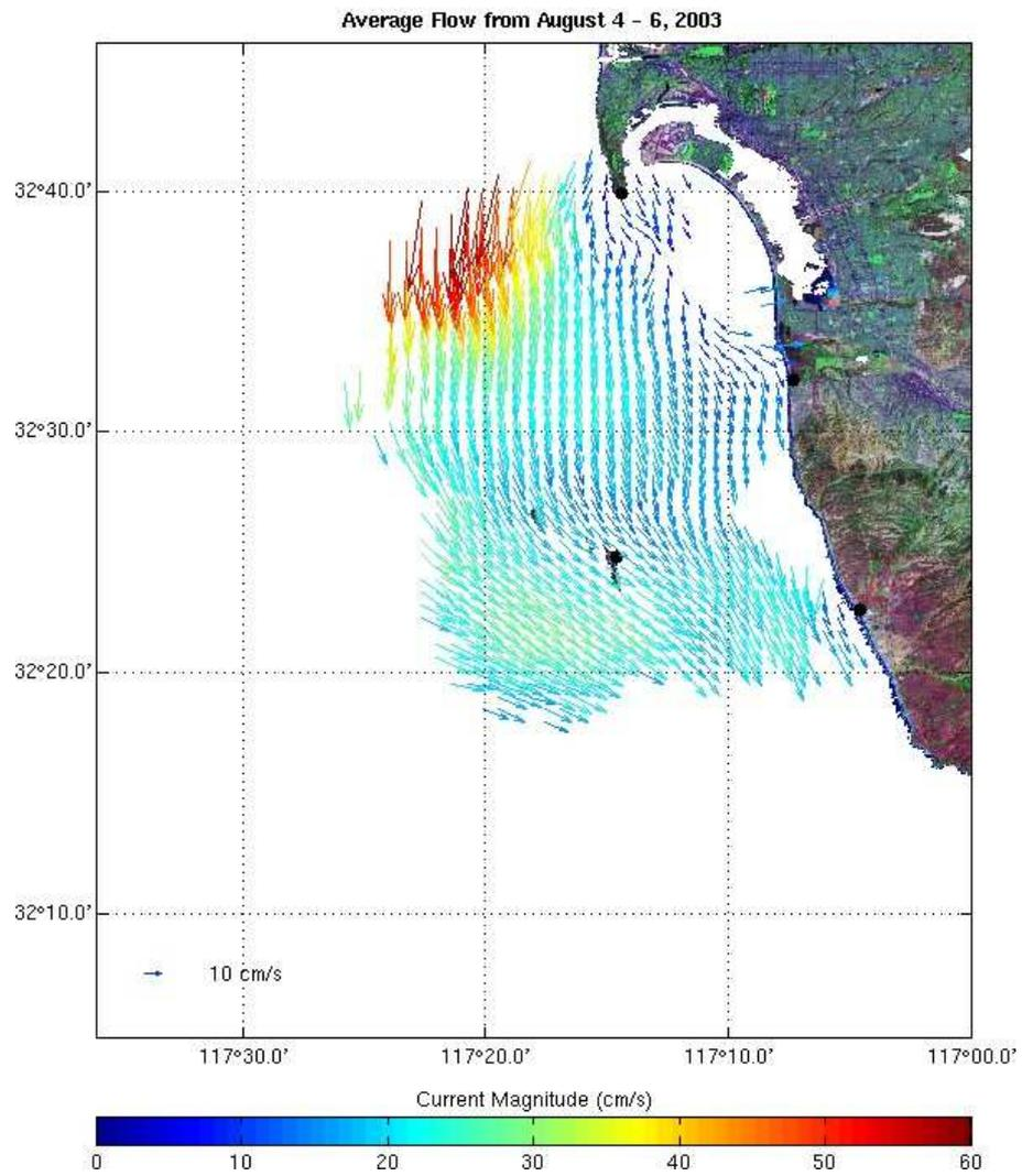
Figure 5.3: CODAR surface currents for 5 August 2003, 0600 GMT. Image from San Diego Coastal Ocean Observing System.
