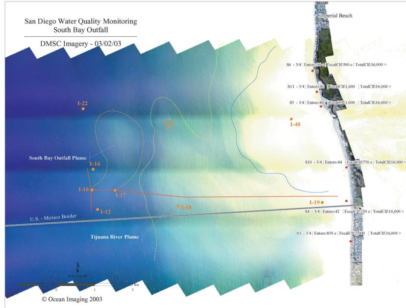
Figure 5.7: Aerial DMSC image from 2 March 2003 showing plumes from both SBOO and Tijuana River. Nearest sampling locations have been overlaid to show relationship between plume boundaries and monitoring stations. Image Copyright *Ocean Imaging*, 2004.
