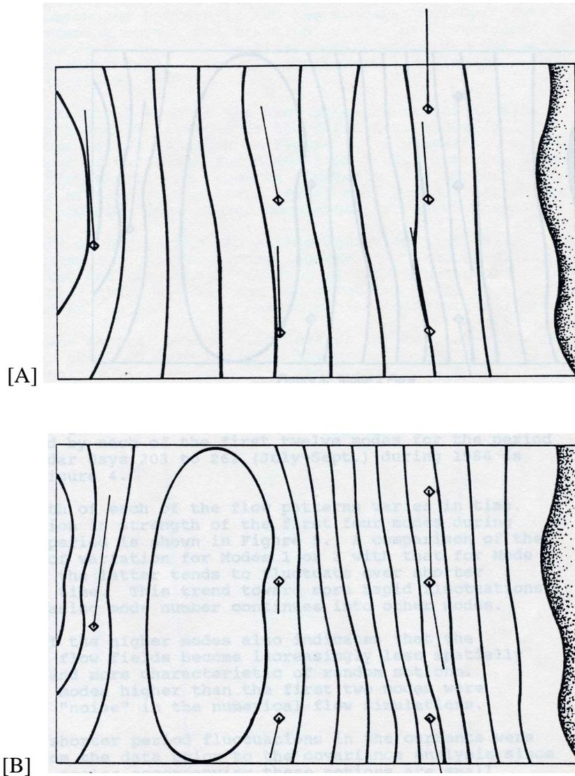
Figure 4.4: Dominant current modes in the South Bay area: A) Mode 1, alongcoast flow. B) Mode 2, shear flow. Vector tails point in direction of flow. Tail lengths proportional to velocity. Flow direction reversals occur with both modes. The dominant direction during the TOES study was downcoast (southwest) for Mode 1, and counter-clockwise for Mode 2. From *Hendricks & Christensen, 1987*.
