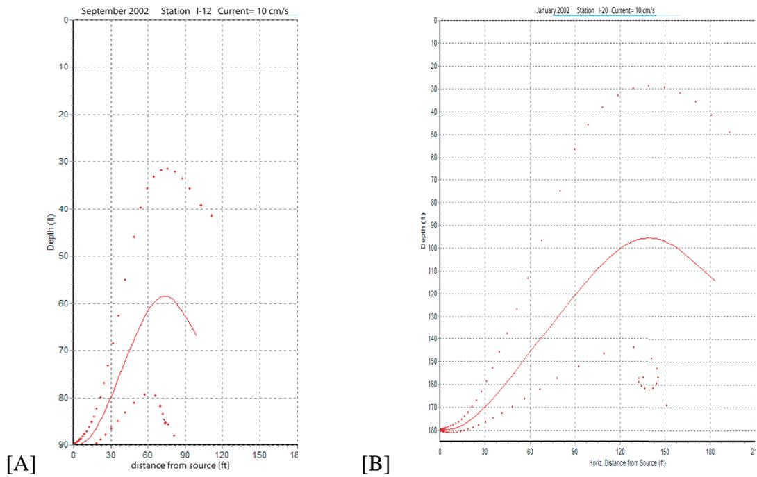
Figure 5.9: Predicted plume heights using CTD profiles for September 2002: A) Station I12, near outfall. B) Station I20, 180 ft depth. Solid red line is plume center, dotted line is boundary.
