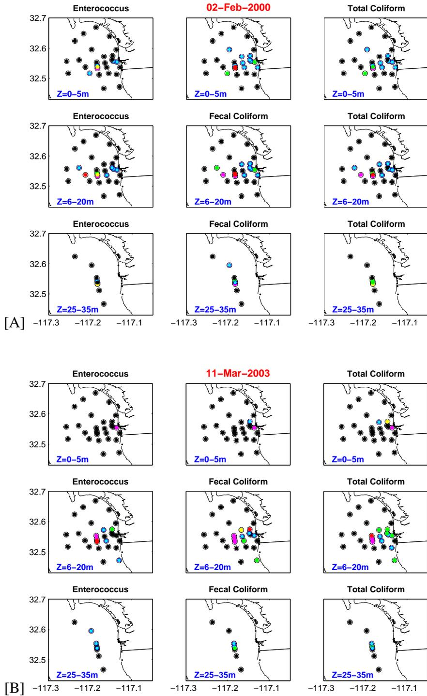
Figure 5.4: Bacterial sampling results showing merging between outfall and river sources: A) February 2000 CTD survey, B) March 2003 CTD survey.
