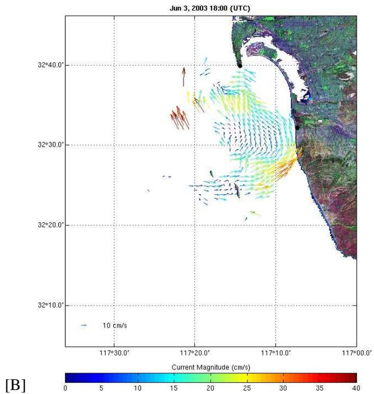
Figure 4.6: Surface currents from CODAR, 2003: A) 3 June, 06:00 GMT. B) 3 June, 18:00 GMT. Images from San Diego Coastal Ocean Observing System.
