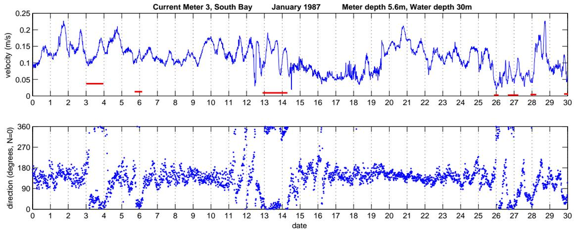
Figure 4.2: TOES current meter data from January 1987 at station C3 in 27 m water depth, 5.6 m current meter depth. Upper panel: current velocity; lower panel: current direction. “Downcoast” is approximately  $160^\circ$ . Red lines indicate periods of flow reversal from down-coast to upcoast.
