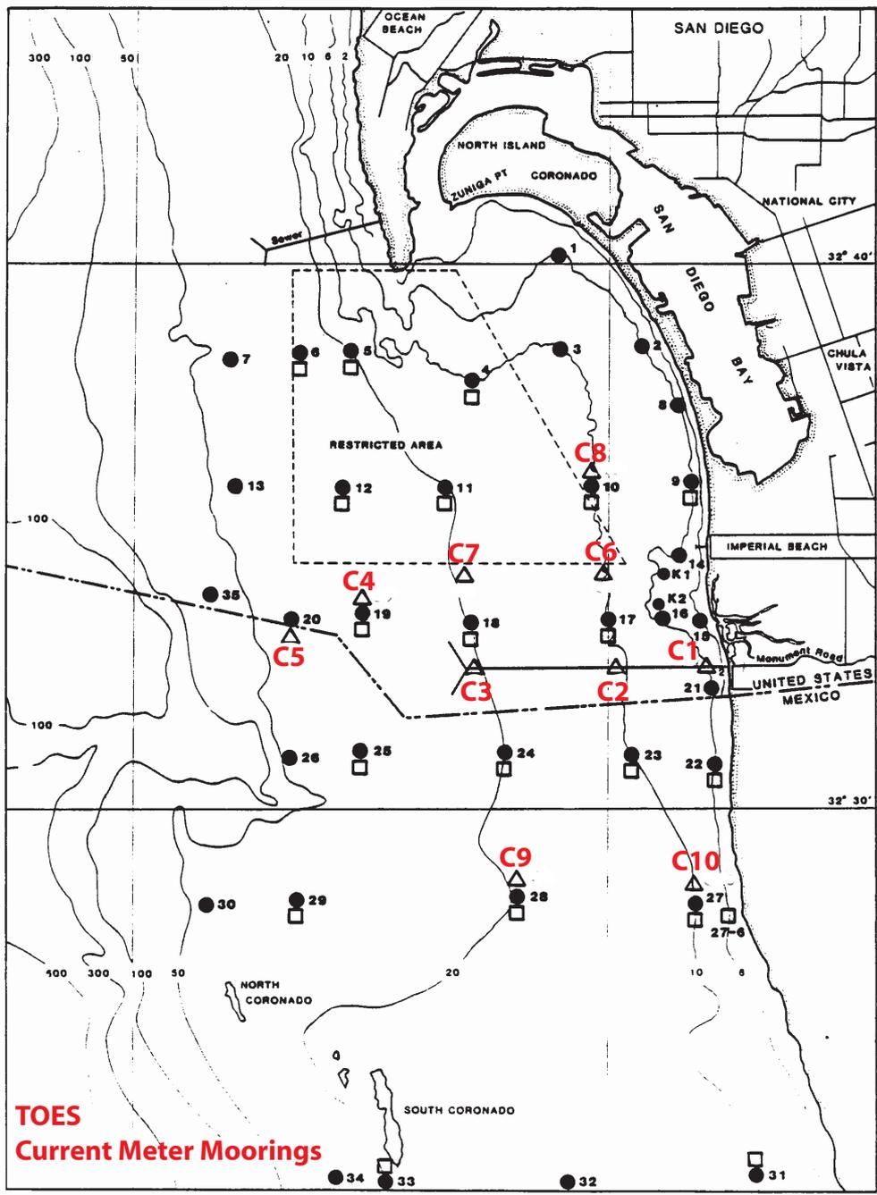
Figure 4.1: Map of TOES current meter stations for Phases I-II (red labels). Circles with small black labels indicate water column sampling stations.
