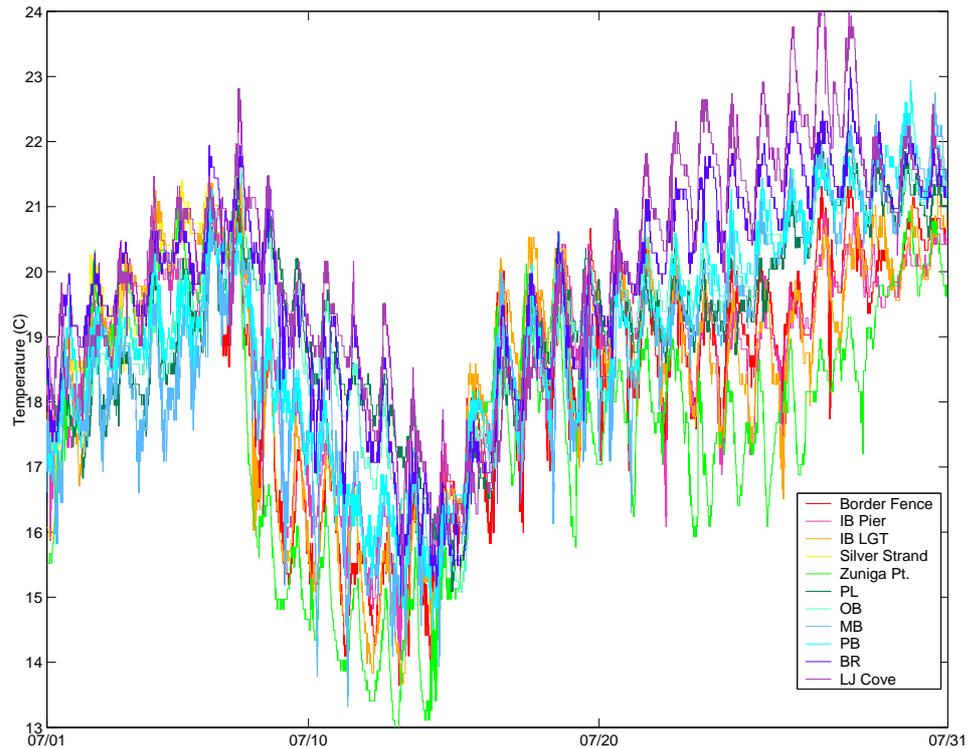
Figure 4.17: High-frequency record of surface temperature at nearshore thermistors in July 2001 (sample interval of 2 minutes).
