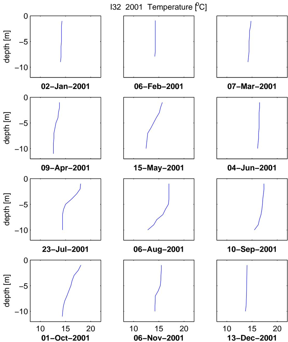
Figure 4.10: Temperature profiles from monthly ocean monitoring CTD surveys, 2001, at station I32 near Imperial Beach .
