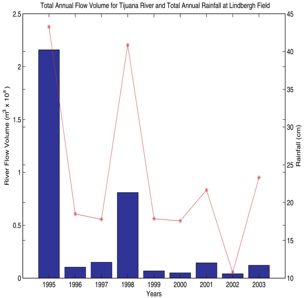
Figure 6.1: Total annual rainfall and river flow for 1995 through 2003. Rain data (red asterisks) are obtained from Lindbergh Field and river data (blue bars) are obtained from IBWC gauge at US-Mexico border.
