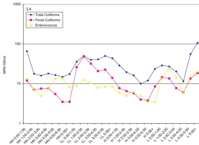
Figure 6.14: Synthesized tidal cycle in bacteria values. Median FIB values (with 3-point running mean smoothing) as a function of the time at which observations were obtained relative to high and low tides. A) Station S10 and B) Station S4.
