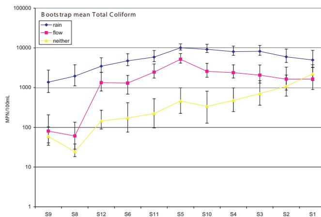
Figure 6.6: Median bacterial levels at each station during rain, flow or neither conditions. Range bars indicate the 95% confidence intervals. A) Enterococcus, B)Fecal Coliform, C) Total Coliform.
