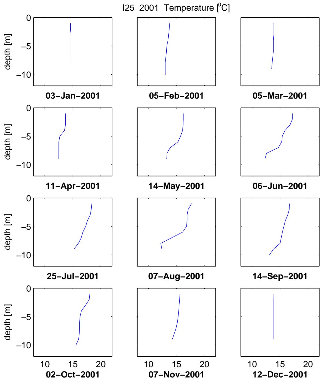
Figure 4.11: Temperature profiles from monthly ocean monitoring CTD surveys, 2001, at station I25 in the Kelp Beds.
