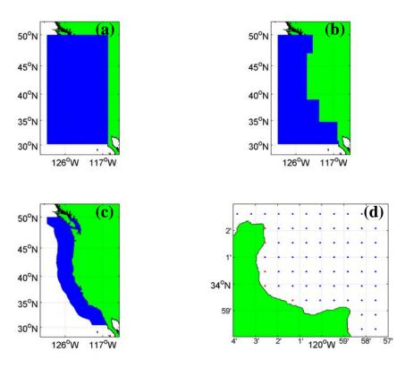
**Figure 1.** The Equidistant cylindrical grid blank for the U.S. West Coast is shown in panel (a). The same grid, after initial gross point elimination is shown in panel (b). Panel (c) shows the grid after points falling over land and outside of the 300km boundary have been removed. Grid points shown in red in panel (d) indicate points that were eliminated from the northeast region of Santa Rosa Island due to their close proximity to land (within 0.5 km).
