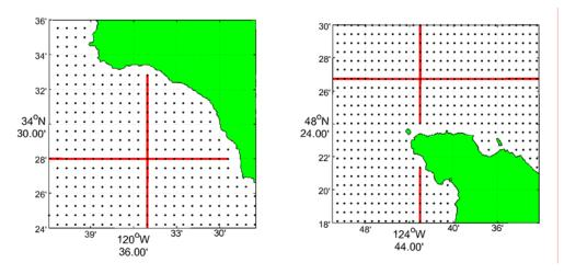
**Figure 3.** Images of the same region show in Figure 1 for the US West coast grid based on an equidistant cylindrical projection. Vertical resolution is constant throughout the grid at 1 km while horizontal resolution increases from 1 km at the southernmost latitude  $(30.25^{\circ} \text{ N})$  to 0.75 km at the northernmost latitude  $(50^{\circ} \text{ N})$ . Arbitrary grid lines highlighted in red show orthogonality is preserved throughout the grid.
