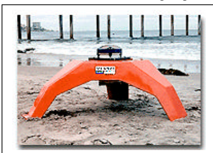
Figure 3. Photograph of what the bottom mounted acoustic current profiler looks like. The profiler will be fixed to the seafloor approximately 300 feet offshore of the I.B. pier.
