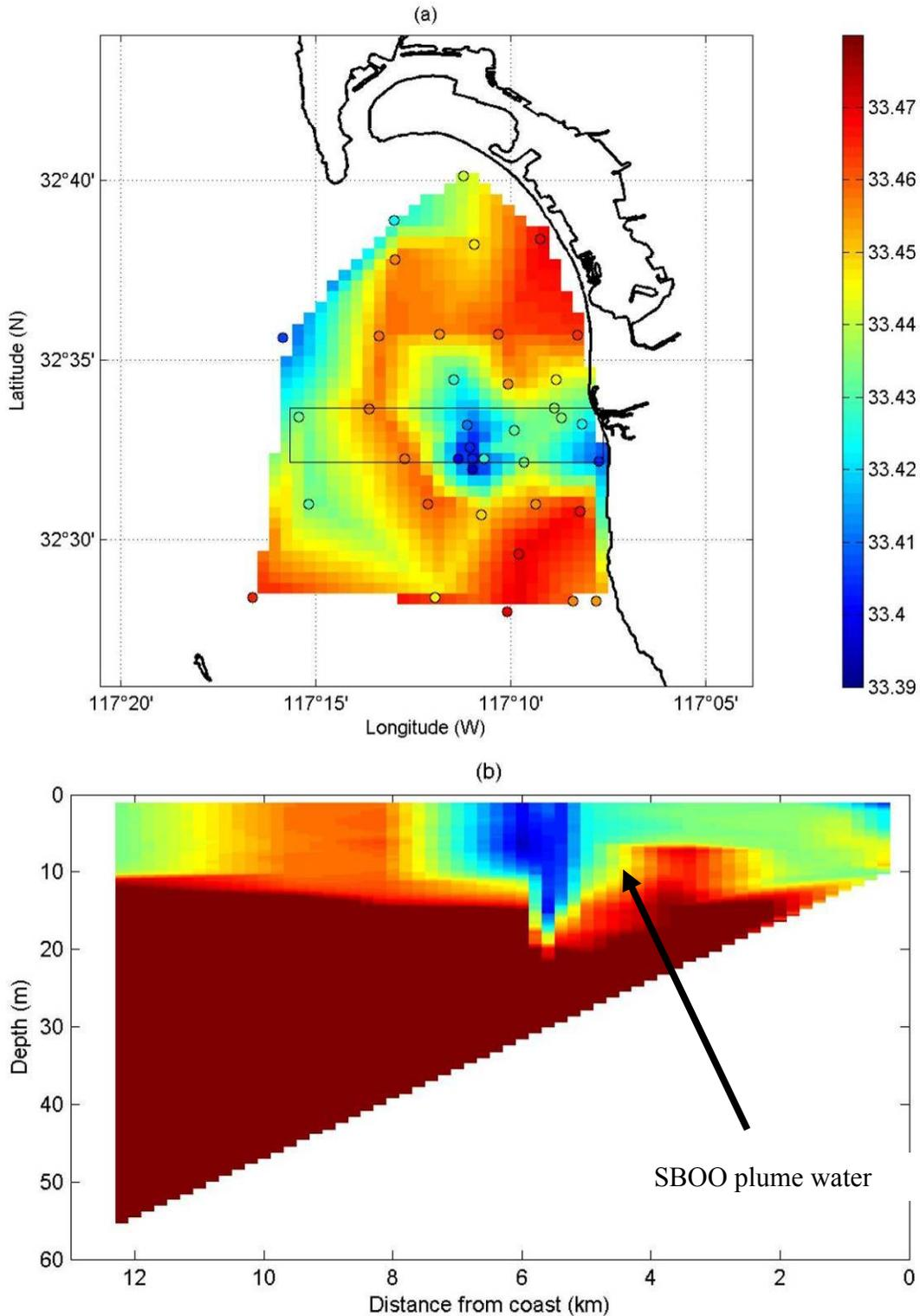
**Figure B.8 Surface Salinity and Ocean Vertical Section – January 16-17, 2008**
