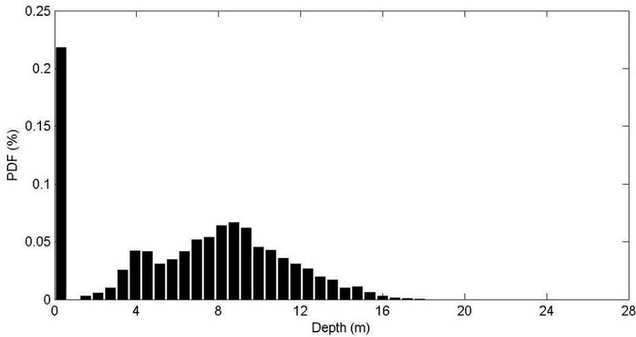
**Figure D.15 SBOO Discharge Plume PDF**
