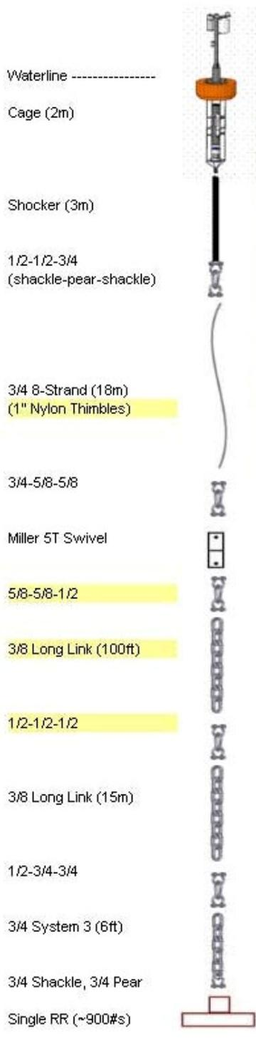
**Figure D.3 SBOO Buoy Mooring Diagram**
