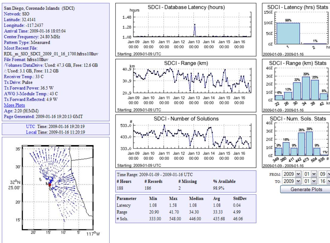
**Figure E.2 HF Radar Diagnostic Utility**
