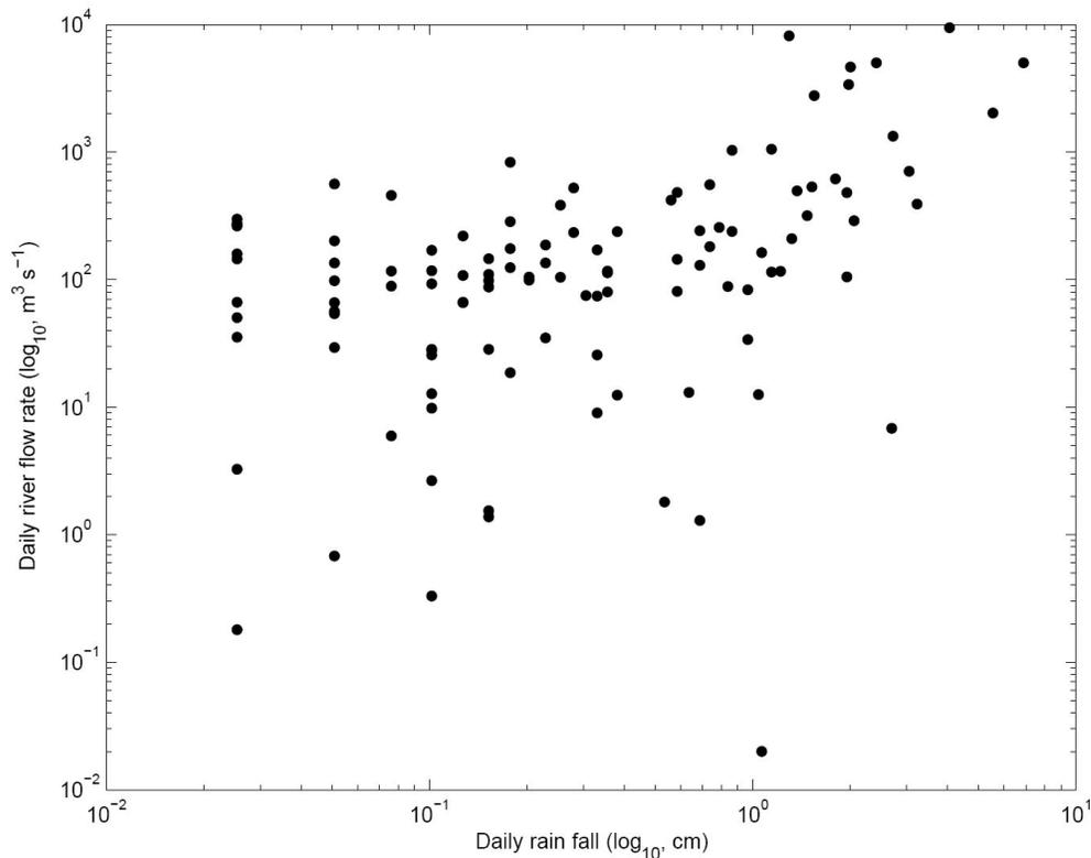
**Figure E.5 Tijuana River Gauge Flow Rate**
