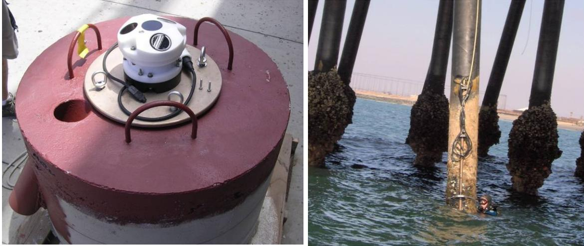
**Figure D.4 Acoustic Wave and Current Profiler**
