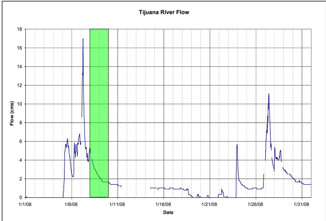
Figure C.8 Tijuana River Flow during January 2008 (sampling dates shaded)
